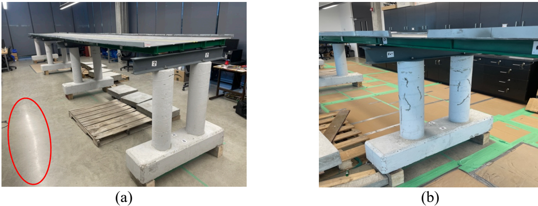
Figure 27. Mitigation of reflective floor surfaces in the indoor lab (a) shows the reflective floor surface (b) shows coverage of reflective surfaces by putting boxes on the floor.
