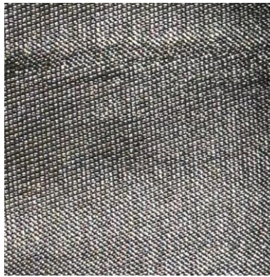
Figure 3.4 Woven Geotextile from Polypropylene Monofilaments: GT-2
