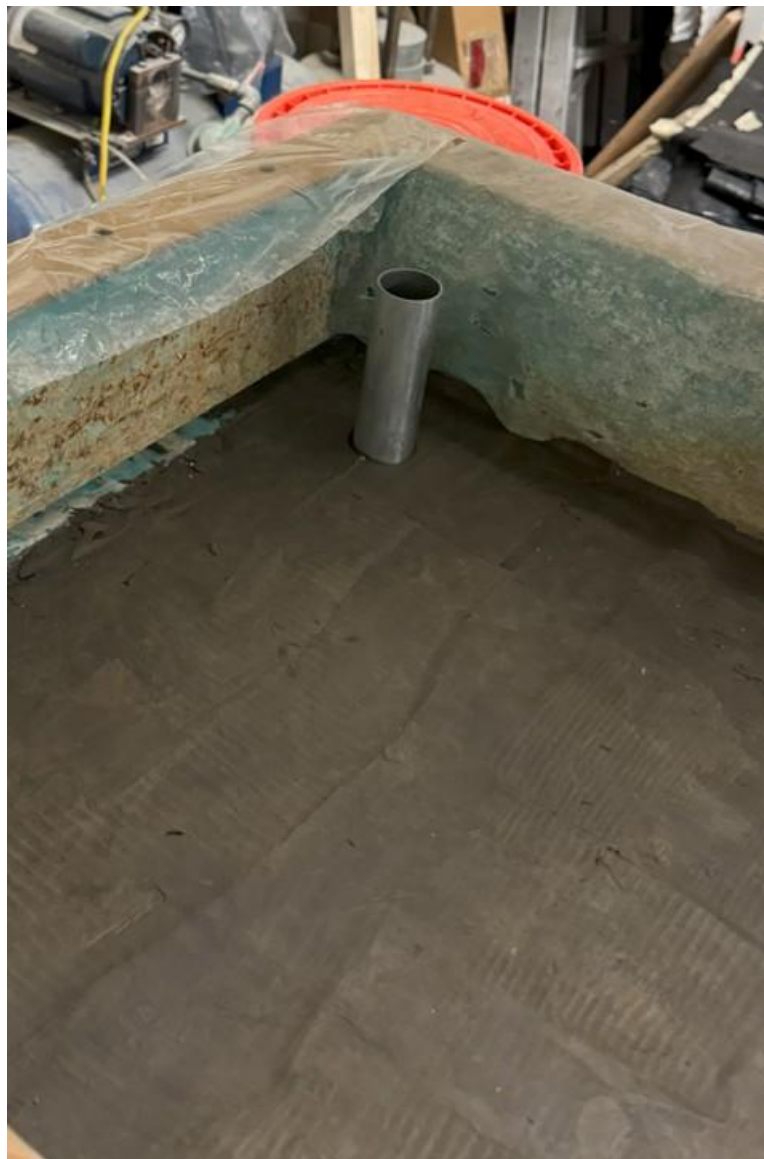
Figure 3.13 Core sample for measuring unit weight of clay upon compaction.
