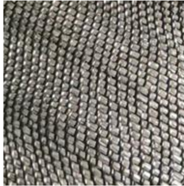
Figure 3.3 Woven Geogrid from Polypropylene Yarns: GT-1
