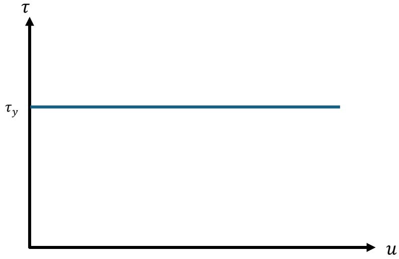
Figure 2.7 Interface Shear of Soil-Geosynthetic Model. (Zornberg et al., 2017)
