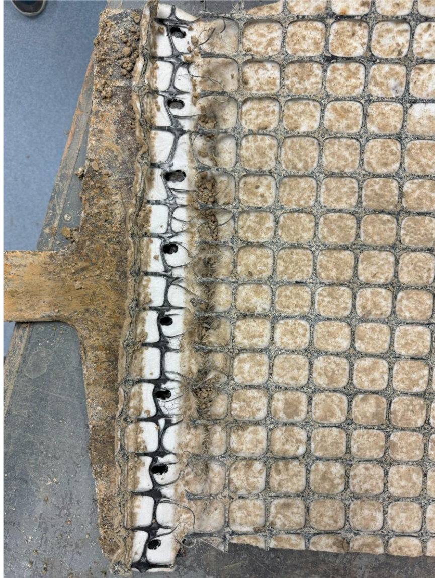
Figure 4.2 Failure of GGC-1.
