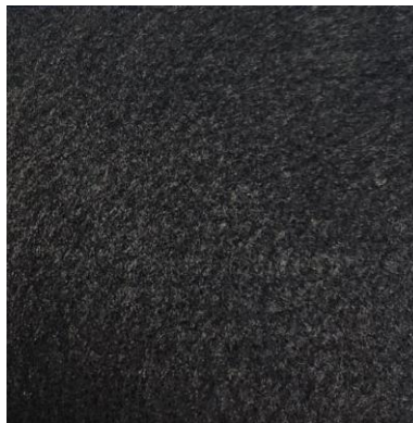
Figure 3.5 Nonwoven Needle Punched Geotextile from Polypropylene Fibers: GT-3
