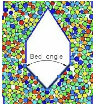
Figure 3-9 Bed angle under the air duct
