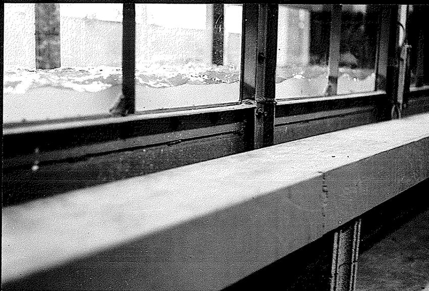
ILLUSTRATION VI: The water surface during a test. The waves shown were generated by a wind velocity of 30 feet per second. The depth of water is 0.4 feet.
