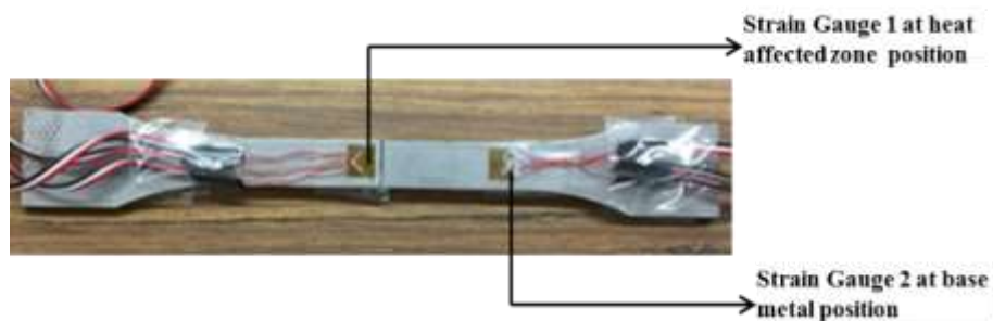
Figure 20: Strain Gauge Location on ASTM Standard Specimen
