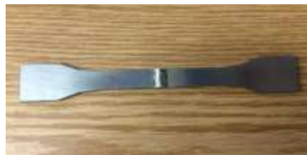
Figure 10: ASTM Standard Arc Welded Specimen
