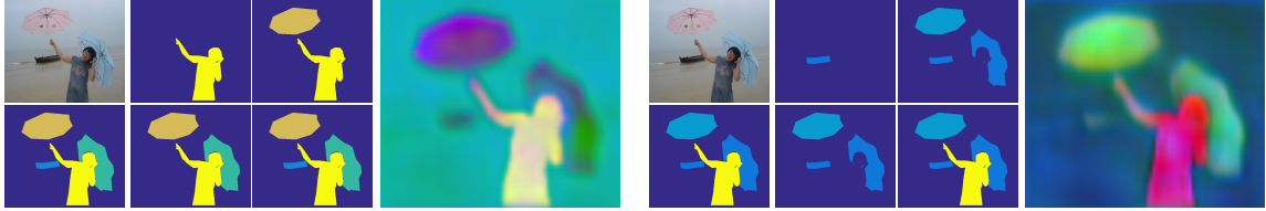
Figure 4.8: Visualization of Principal Component Analysis (PCA) for the final prediction stack (NRSS) for both the relative (left set) and the absolute (right set) cases. For each set, the first column shows the image and its ground truth. A selection of ground truth stack slices is shown in second and third column. The top three principal components for our predicted stack is visualized as an RGB column.
