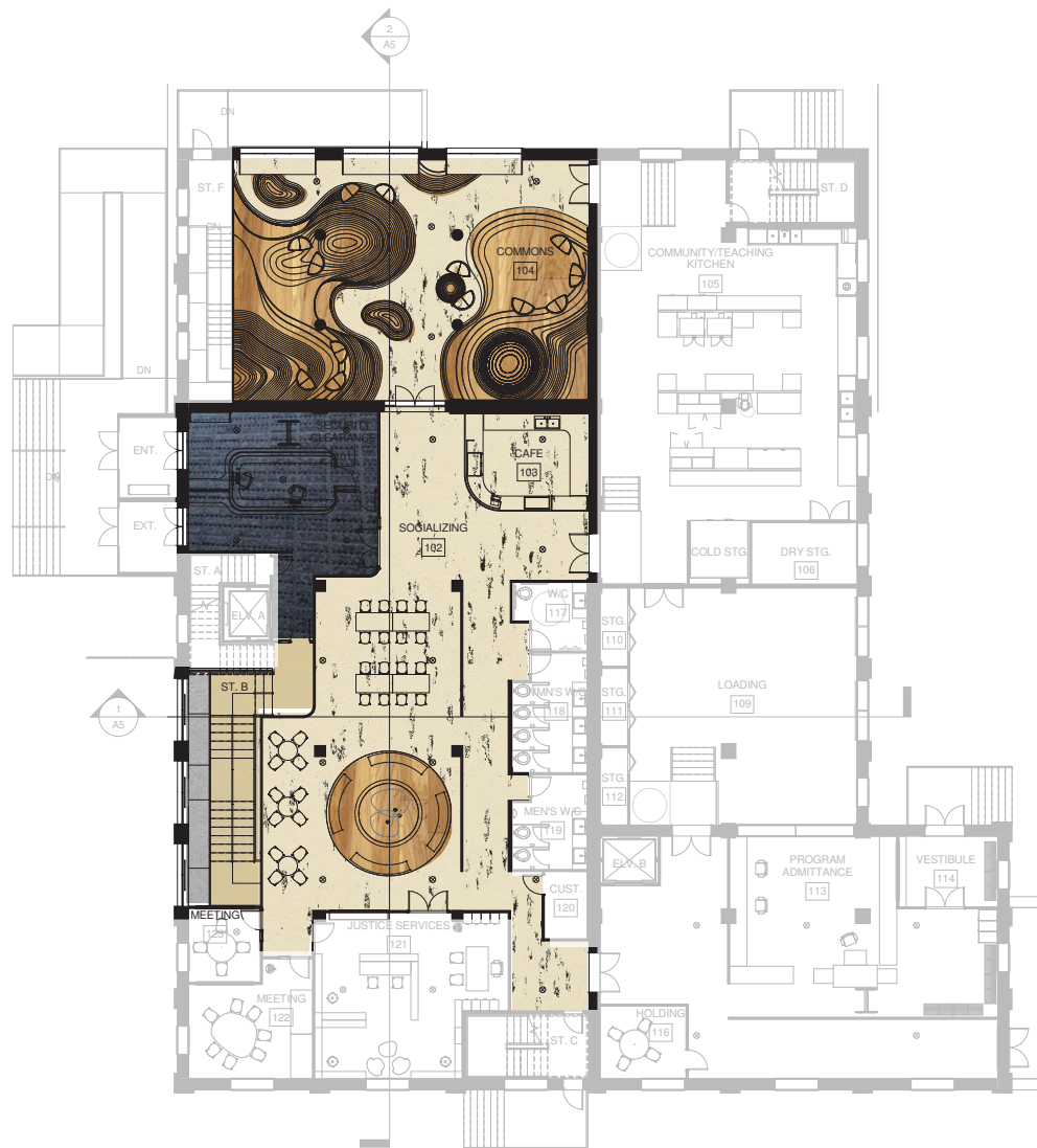
FIGURE 80 - FLOOR FINISH PLAN - GROUND LEVEL
