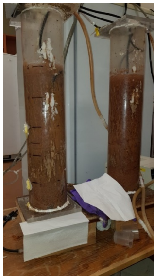
Figure A.1: GSBRS (R1 and R2) in operation.
