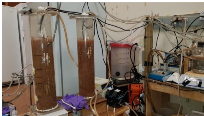
Figure B1. AGS-SBRs (R1 and R2) in operation
