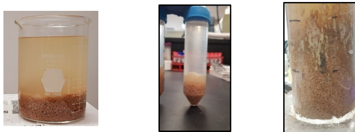
Figure D2. Cultivation of large sized AGS ( \geq 2.5 mm) through the mother SBR under during the treatment of high-strength wastewater
