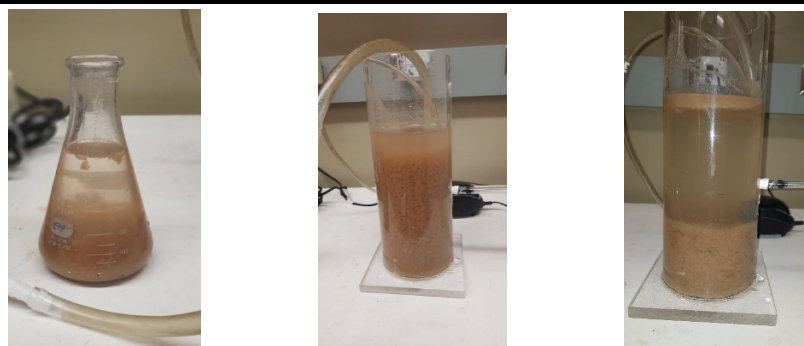
Figure D3.a. Deterioration in the physical properties via continuous P-rich liquid extraction (R2) (significant reduction in granules' size)
