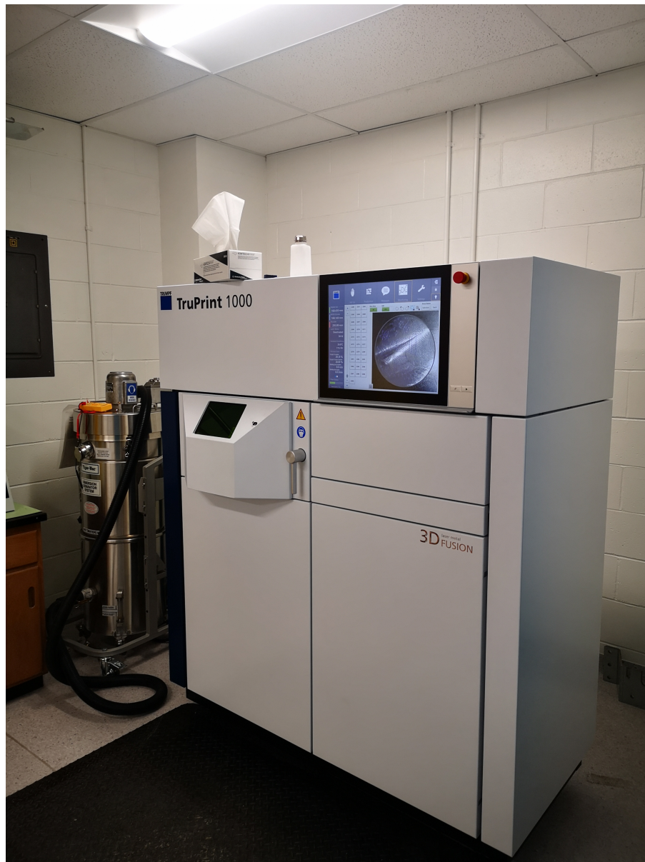
Figure 4.5: TRUMPF TruPrint 1000, the printer used for all additive manufacturing of metals in this project.
