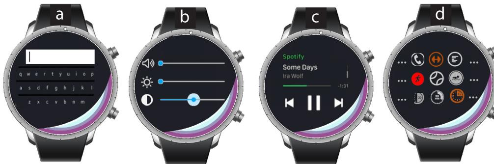
Figure 6.13: a) Each of the three EdgeSelect bands can be used to interact with a three-row virtual keyboard on the smartwatch without blocking the letter while typing. b, c) Using EdgeSelect to interact with sliders such as adjusting settings and navigating through music tracks. d) EdgeSelect can also be used in hierarchical menus for item selection.
