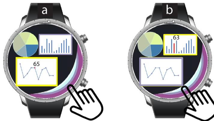
Figure 6.6: a) Interacting with line graph using the Outer-band of interaction area b) Sliding the index finger into the Middle-band to interact with bar chart. Moving from one band to another band changes the highlighted graph to make it easier for the user to identify the graph they are interacting with
