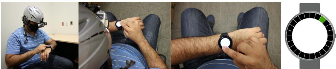
Figure 5.1: Screen occlusion study setup. A camera was mounted to the front side of a helmet to capture images of the finger on a region of the bezel from the user's vantage point. Images were then processed to compute the degree of occlusion.
