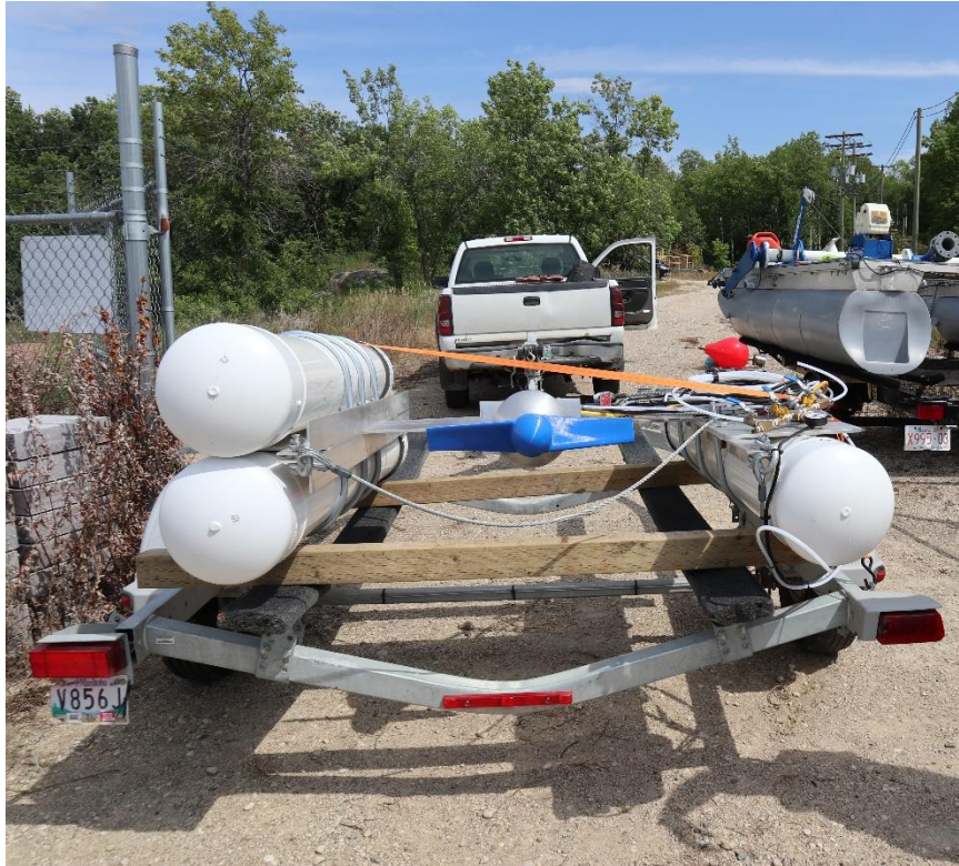
Figure 30: CT-HKT mounted onto a zodiac boat trailer for easy deployment at the CHTTC.
