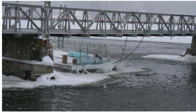
Figure 10: Ice accretion around a near-surface HKT. This can cause structural damages to the HKT. The damage can also cause the floatation system to malfunction or break entirely causing the HKT to sink.
