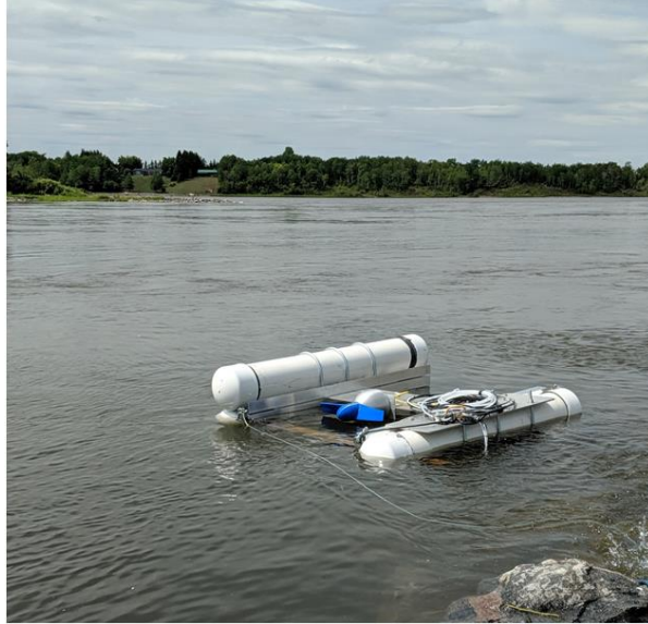
Figure 51: The CT-HKT being launched at the Jackfish Bay. The figure shows both 4X4 beams underneath the HKT as it launched for the first time.
