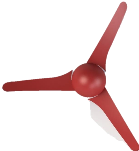
Figure 34: CAD model of the blade used in experiments conducted in the water tunnel by Shahsavarifard et al. Blade was modelled to the nearest millimetre so as to reduce errors in the validation study
