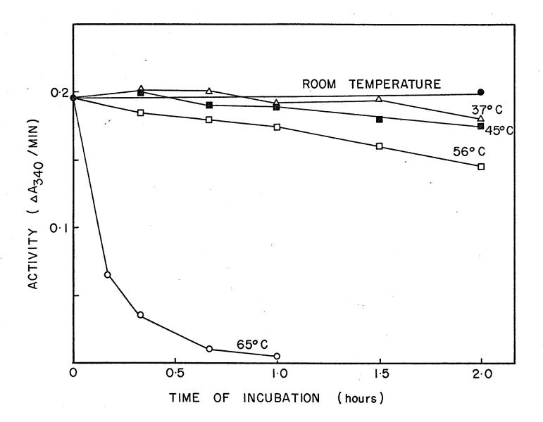
TABLE VI Stability of PFK before and after heat treatment at  $56^{\circ}\mathrm{C}$
