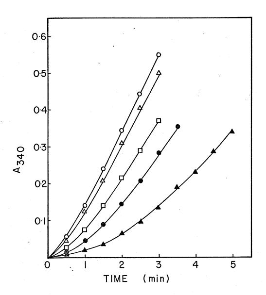
Figure 14. Effect of  $(NH_4)_2SO_4$  on the PFK assay with 4.4 mM ATP. Concentrations of  $(NH_4)_2SO_4$  were: 0 mM  $(\bigcirc-\bigcirc)$ , 5 mM  $(\bigcirc-\bigcirc)$ , and 100 mM  $(\bigcirc)$ . Other assay components were as described in Materials and Methods.
