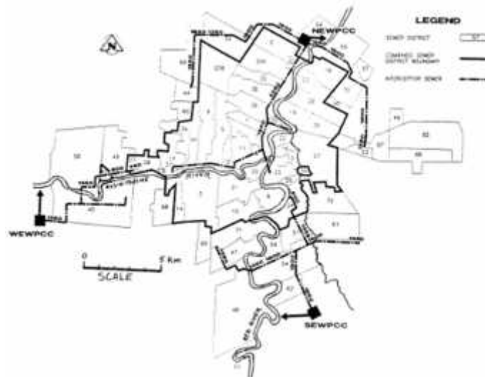
Figure 1.6 Locations of the three wastewater treatment plants within Winnipeg, Manitoba. The North Main Water Pollution Control Centre (NEWPCC) is located in the north end of Winnipeg.
