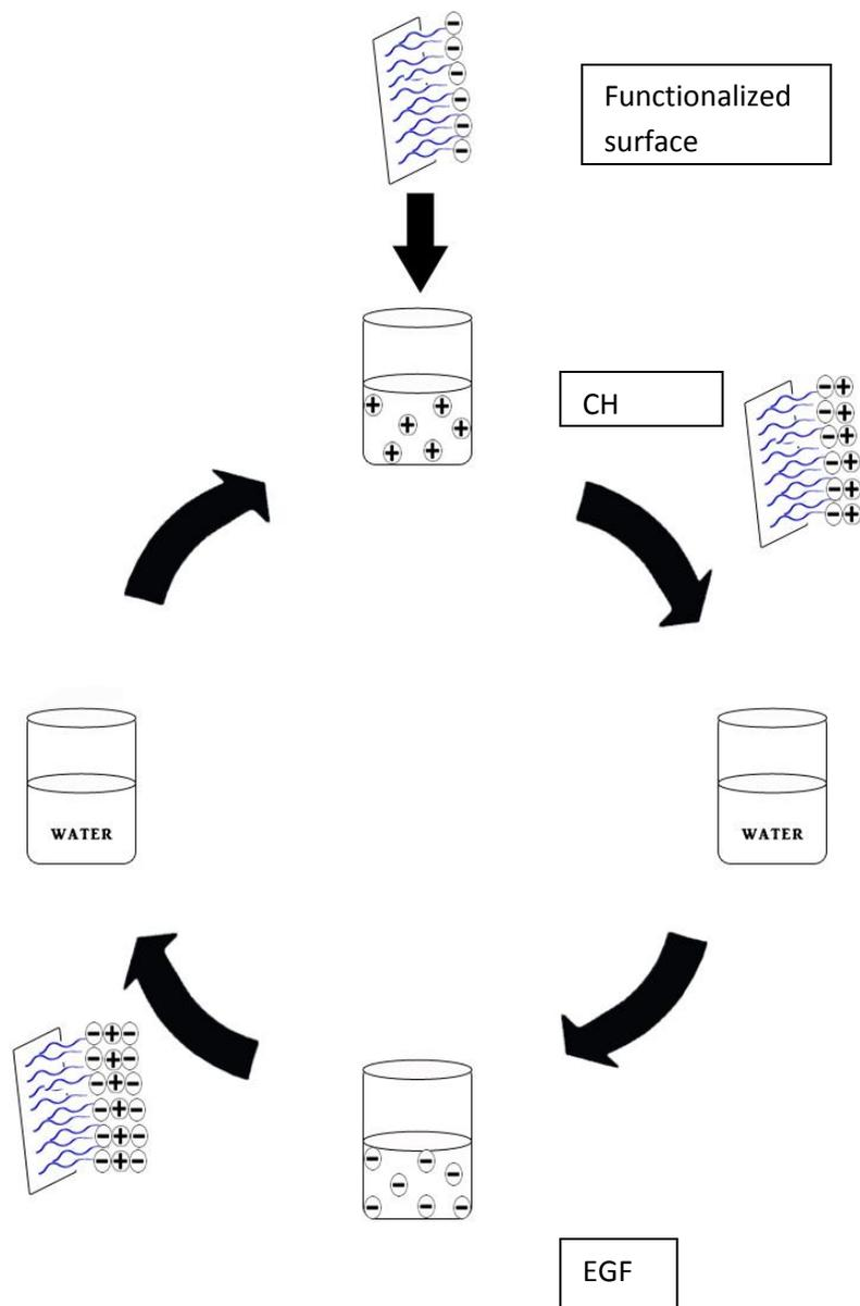
**Schematic Diagram 2:** Illustration of layer-by-layer assembly of polyelectrolytes.
