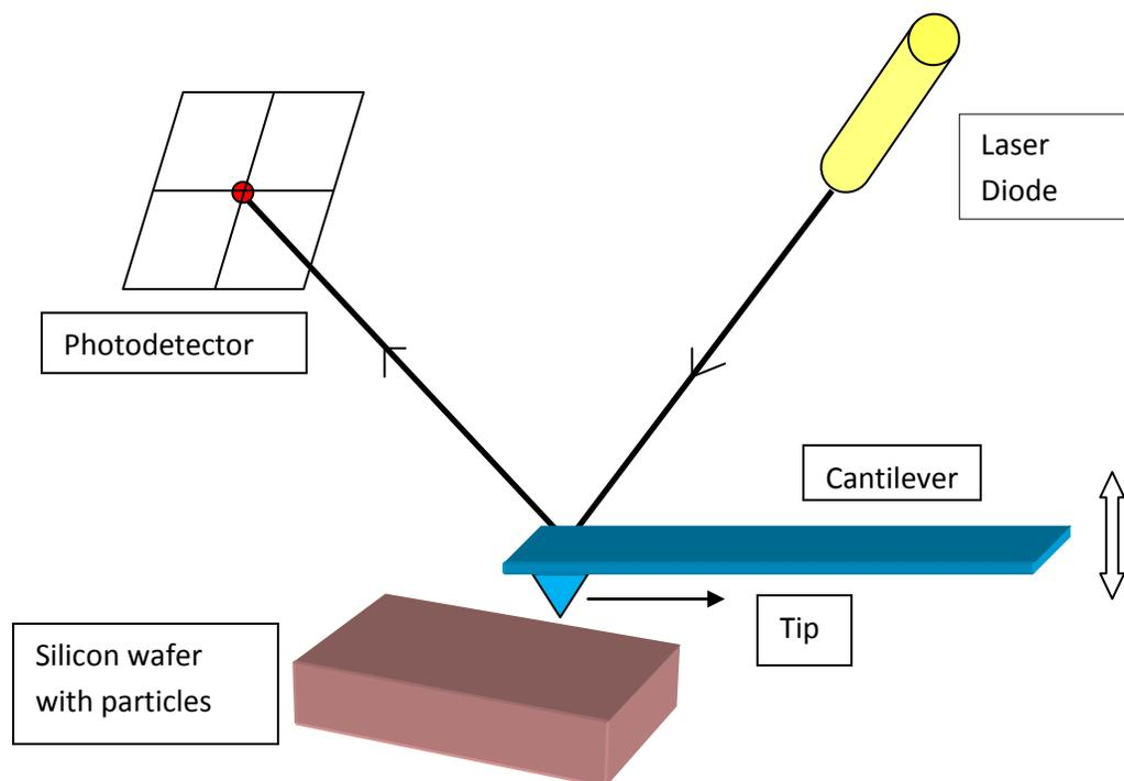
**Schematic Diagram 4:** Working principle of AFM
