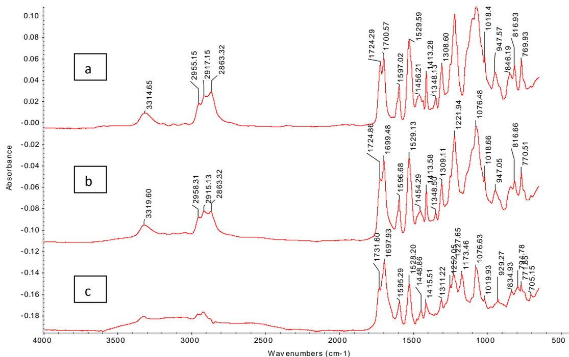
**Figure 2.** FTIR spectra of (a) untreated PU film; (b) PAA modified PU film; and (c) subtraction of (a) from (b)
