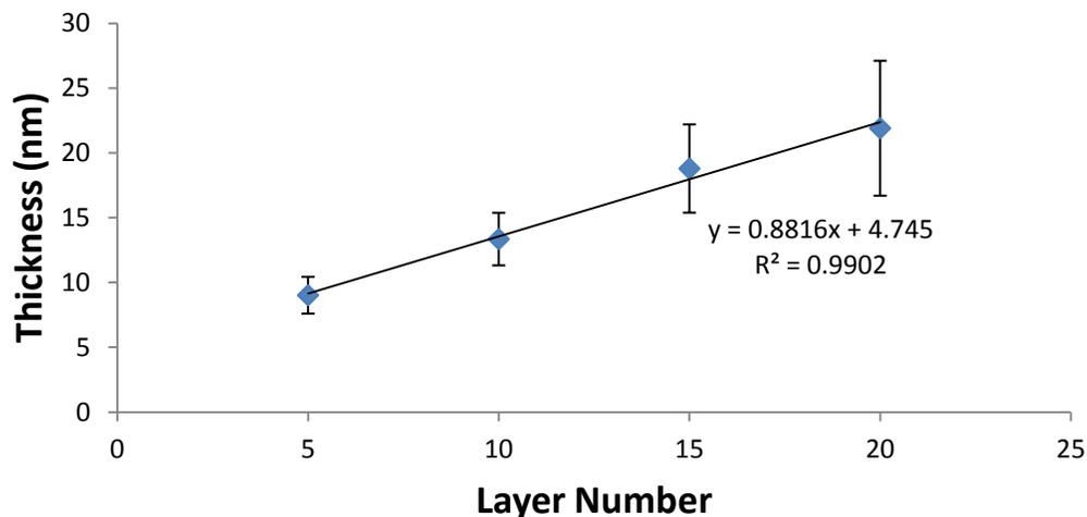
**Figure 5.** Thickness measurements of 20 layers of polyelectrolytes on silicon wafer.
