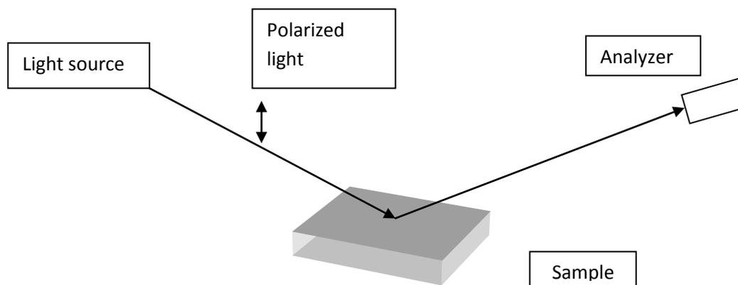
**Schematic Diagram 5:** Mechanism of Ellipsometry
