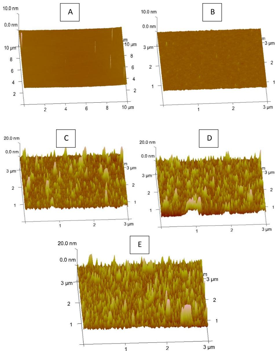
**Figure 4.** AFM images of a) silicon wafer b) modified silicon wafer (a layer of carboxyl group) c) 5 layers of CH/EGF d) 10 layers of CH/EGF e) 15 layers of CH/EGF.
