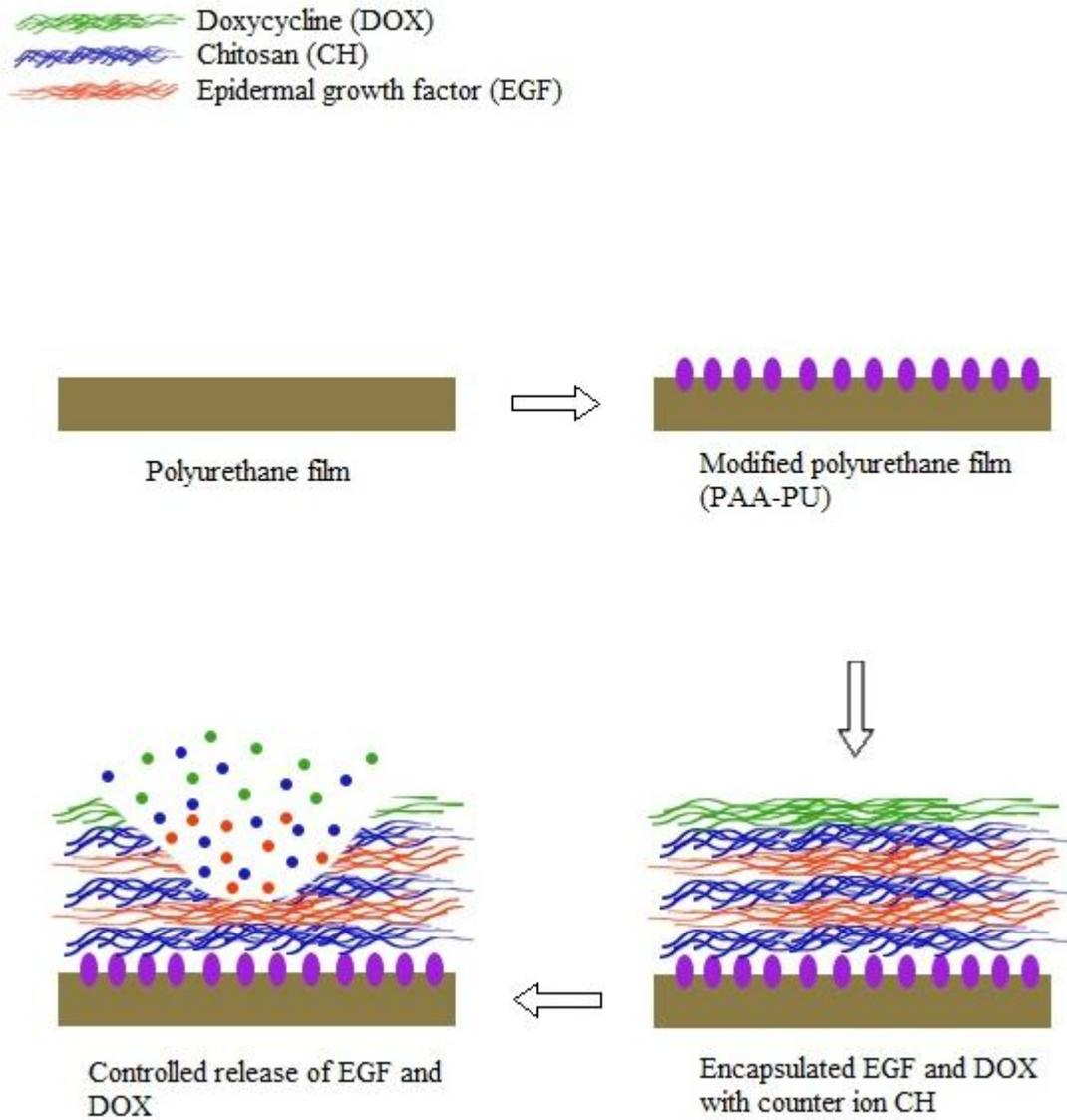
**Schematic Diagram 1:** Schematic representation of experimental design and methodology.
