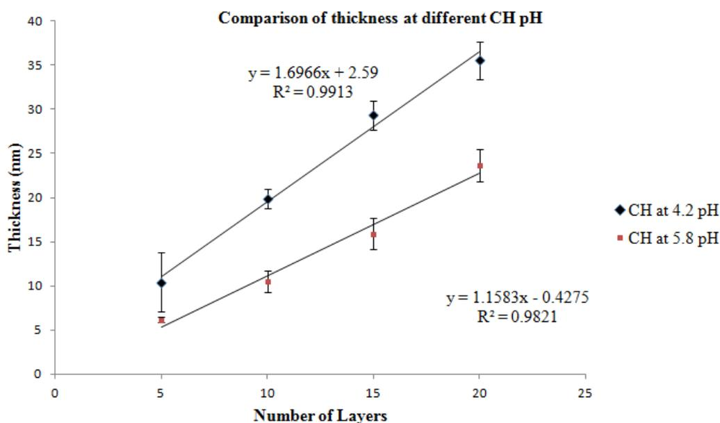
**Figure 13.** Thickness measurements for (CH/DOX)<sub>10</sub> CH at pH 4.2 and pH 5.8.
