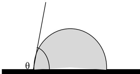
**Schematic Diagram 3:** Mechanism of contact angle measurement.
