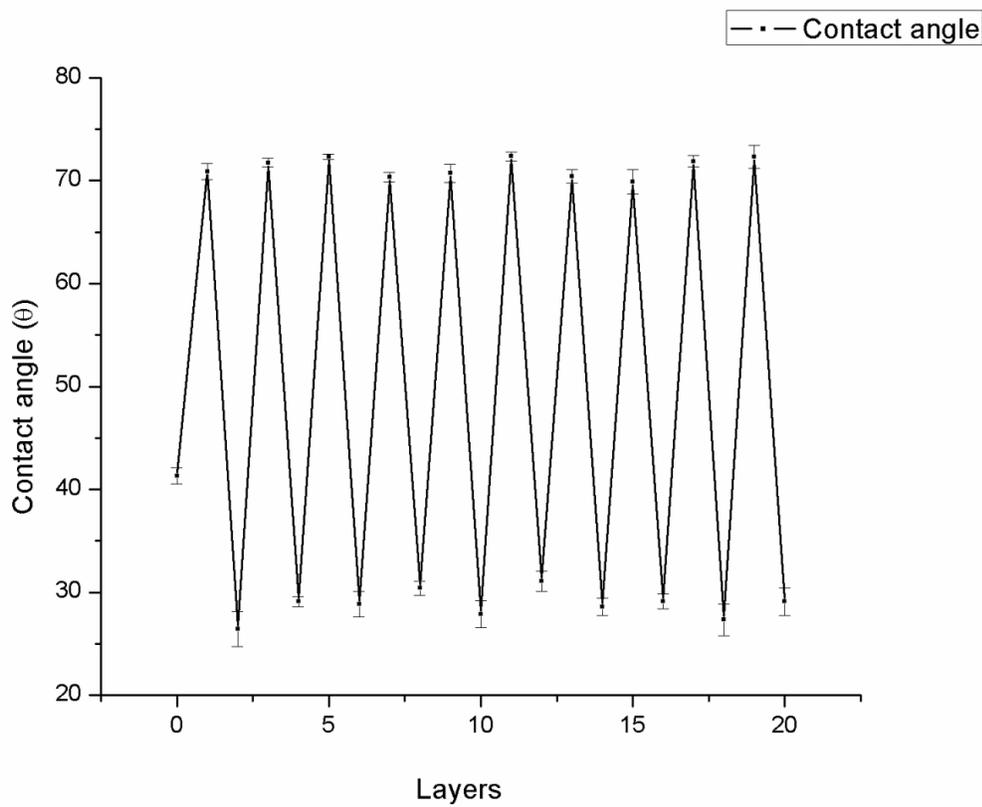
**Figure 11.** Contact angle measurements for CH and DOX on silicon wafer (20 Layers).
