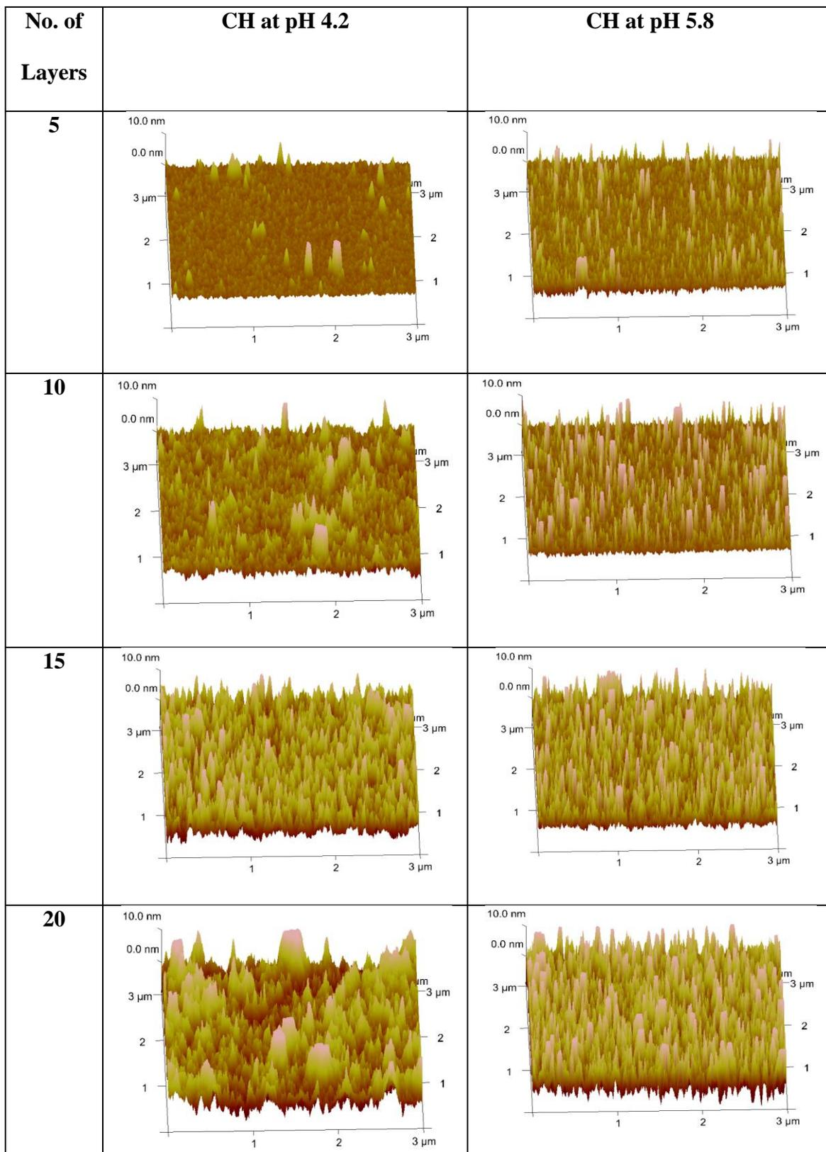
**Figure 12:** Comparison of AFM images analyzed at CH pH 4.2 and pH 5.8.
