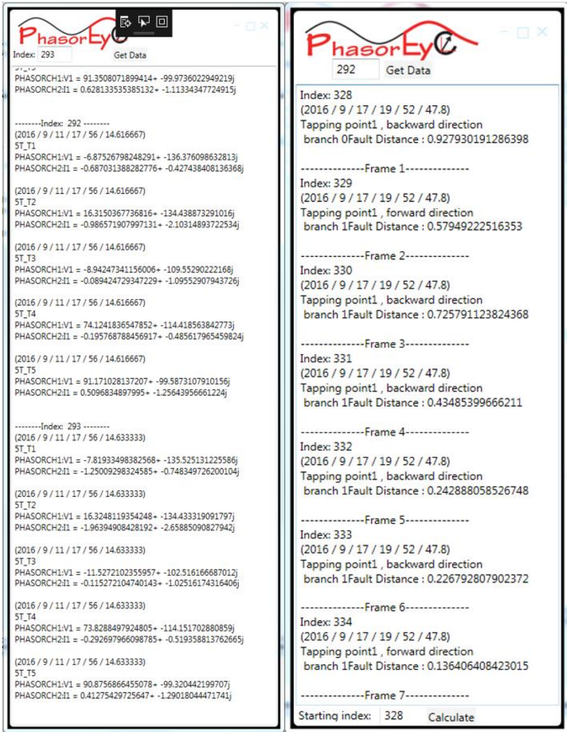
Figure 4.23 Feeding data from data player (left) into synchrophasor measurement-based fault location algorithm (right)
