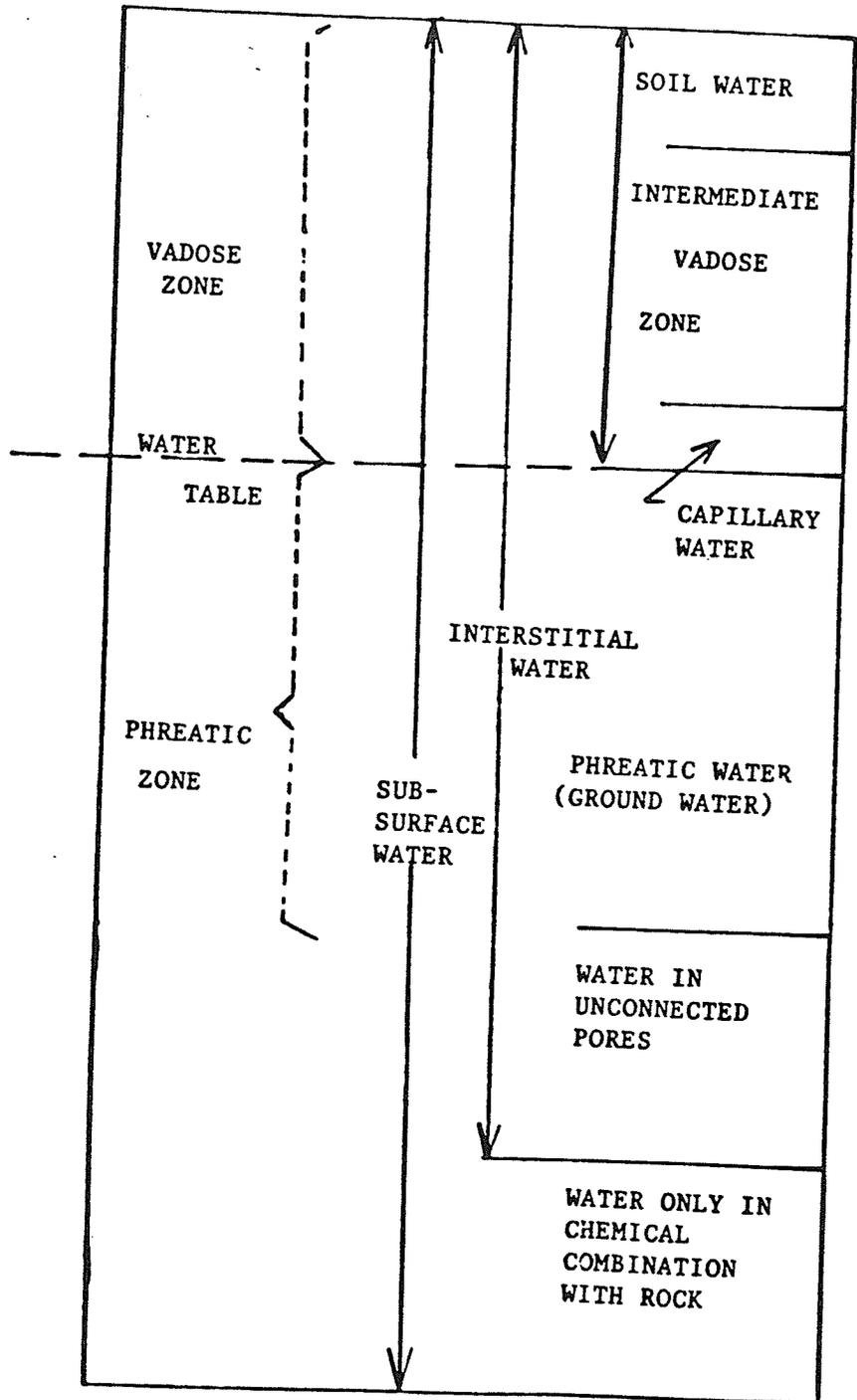
FIGURE 2: CLASSIFICATION OF SUB-SURFACE WATER.
