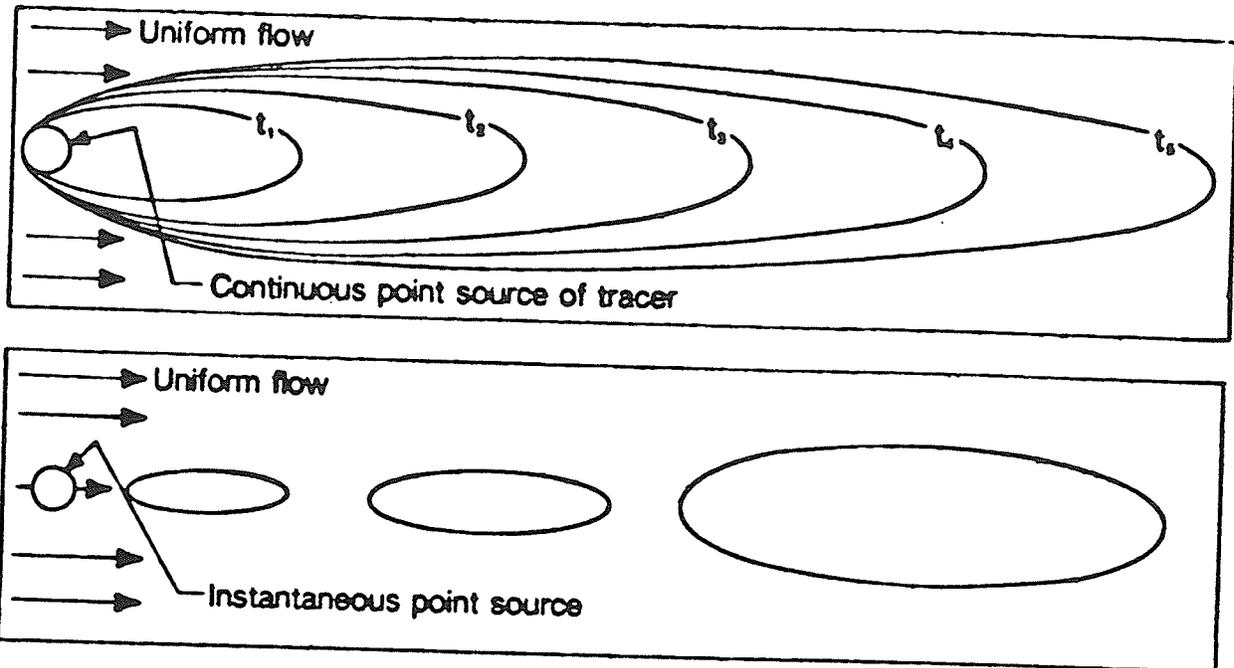
FIGURE 18: SPREADING CHARACTERISTICS OF A TRACER (From Freeze and Cherry, 1979.)
