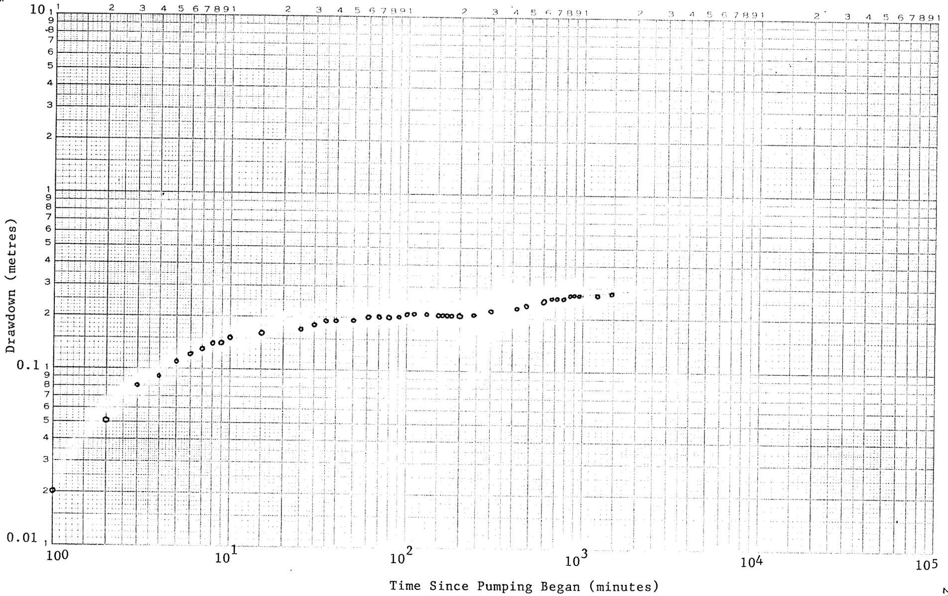
Figure 4: Test Data Plot on LOG-LOG Scale (Data from Table 2)
