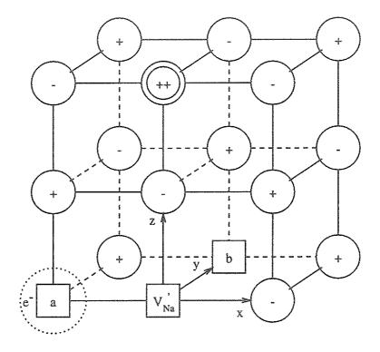
Figure 4.15: The  $(F_2^+)^*$  center: configuration 11
