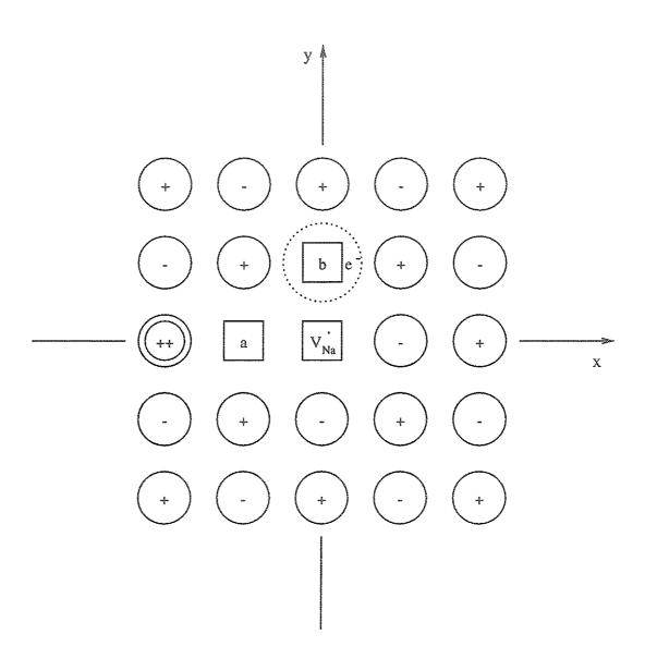
Figure 4.8: The  $(F_2^+)^*$  center: configuration 4
