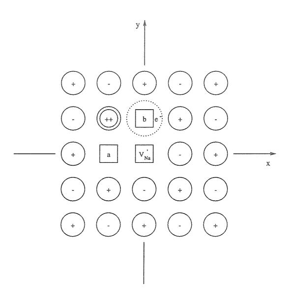
Figure 4.9: The  $(F_2^+)^*$  center: configuration 5
