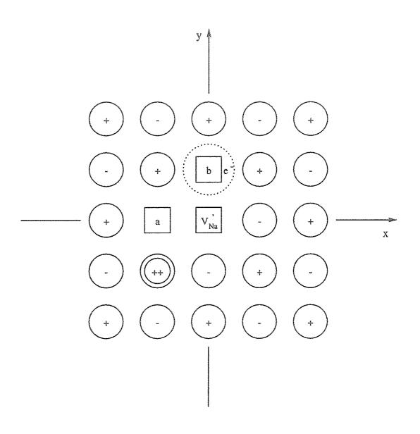
Figure 4.7: The  $(F_2^+)^*$  center: configuration 3
