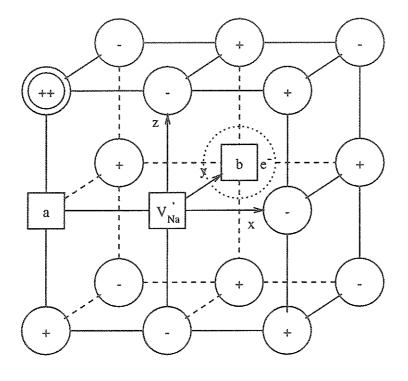
Figure 4.13: The  $(F_2^+)^*$  center: configuration 9
