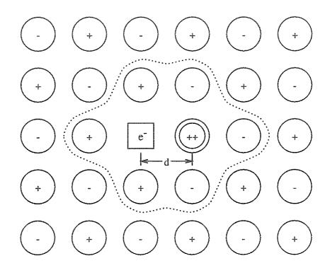
Figure 4.5: The nearest-neighbor cluster for deriving F center-Mg<sup>2+</sup> interaction
