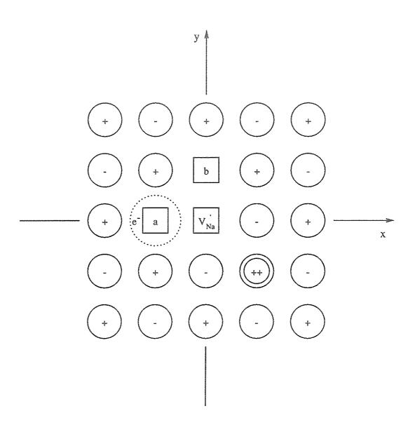
Figure 4.6: The  $(F_2^+)^*$  center: configuration 2
