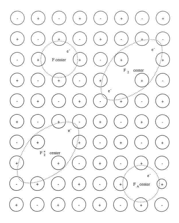
Figure 2.1: Common F-type centers in ionic crystals
