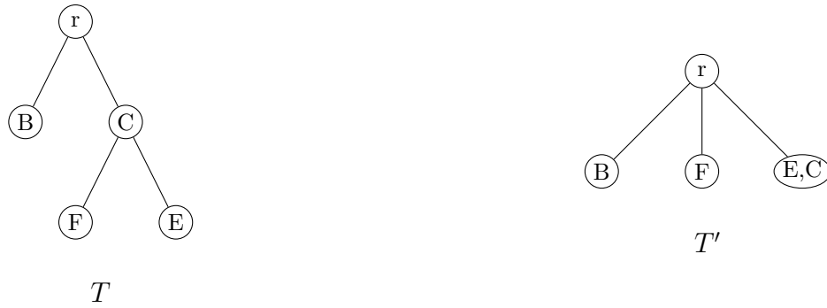
Figure 4.4: Rearrangement between existing nodes resulting in node removal: The tree T' is the tree T after moving the label C to the node labeled E . The rearrangement of the label C , as shown above, removes its original node and changes the historical contents of the nodes labeled F and the label set of the node labeled with E .
