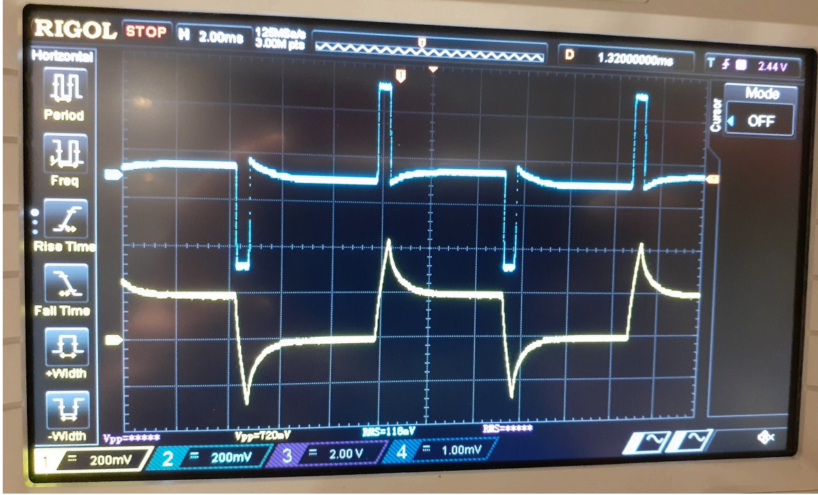
Figure 5.3: shows the switching of the quadrupole coil with DOS 25 V, 80 A. The shaped input signal with an overshoot and undershoot is given to the Matsusada. The exponential feature in the input signal is to counteract the exponential response due to eddy currents. The blue waveform in this figure is the arbitrary waveform, and the yellow curve is the current flowing through the quadrupole coil observed from the monitor channel of the power supply.
