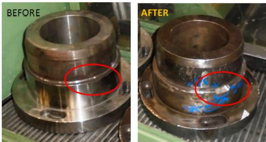
Figure 7: Before and after pictures of the modified chuck with the new cut-out slot [7].
