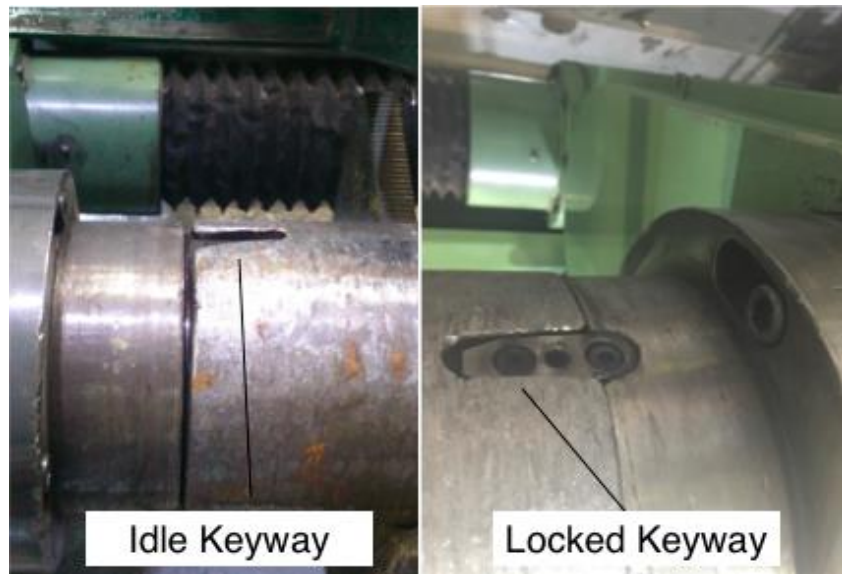
Figure A.3: Idle and locked keyways of the core [7]
