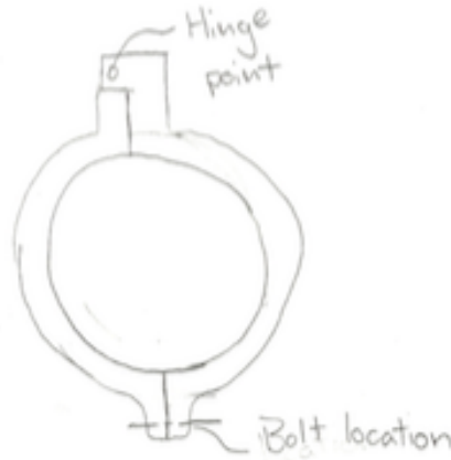
Figure A.10: This image shows a concept for the hinged connection ring used to connect a scissor jack to the splitter and core
