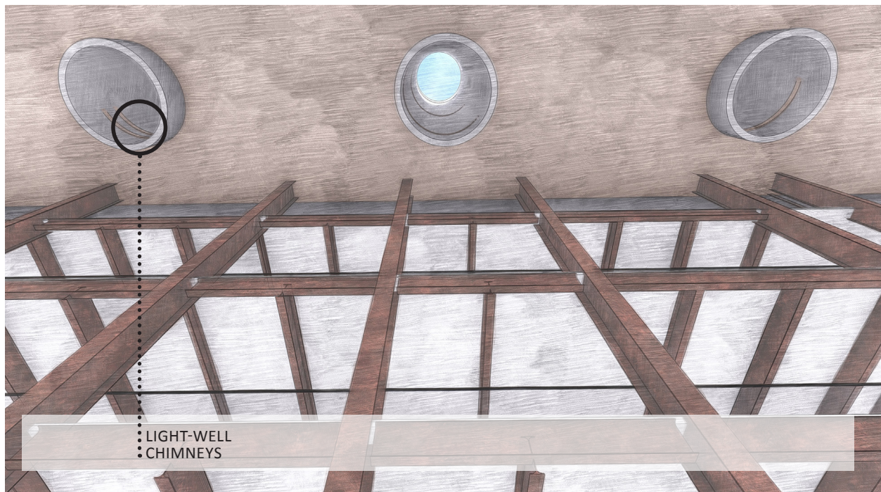
Figure 8.45 Lightwells serve to introduce daylighting, and acts as a metaphor for chimneys and interpret the adaptive re-use of a former coal-powered electricity generation station.
