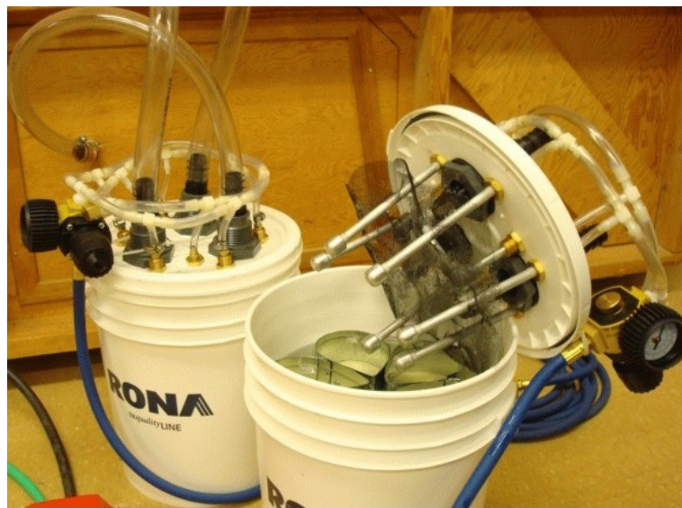
Figure 2.26. Custom-built particle generators for seeding.
