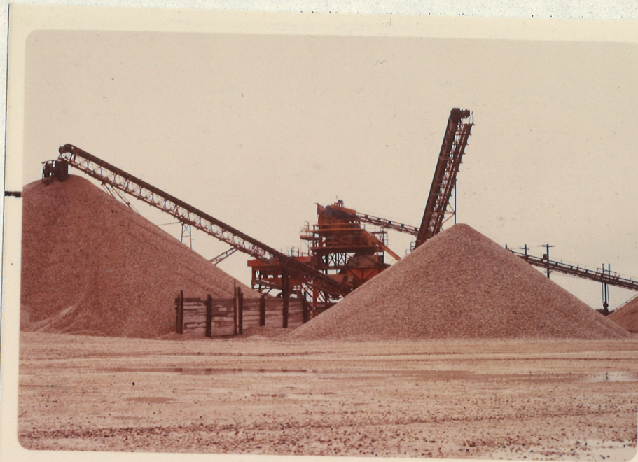
Photo #6: A screening plant, sorting aggregate into stockpiles of various size categories.
