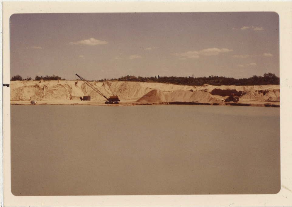
Photo #16: Enormous lakes may be created by mining below the water table. The potential for ground water disruption or contamination is high.
