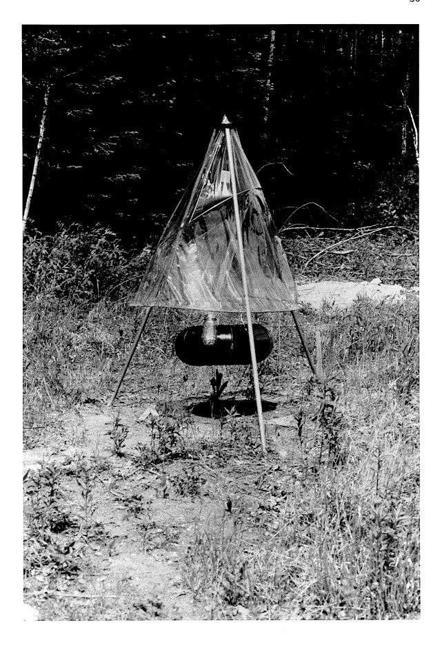
Figure 4. The design of the Manitoba Horse Fly Trap used in 1984. The plastic and aluminum pipes were from the same design as used in 1983. Glossy, black spheres approximately .61 m in diameter (as those used by Thorsteinson et al., 1964) were used for visual attractance. A small container was placed at the apex of the trap, into which the flies were collected.
