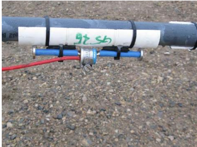
Figure 3.5 - Typical Strain Gauge Installation
