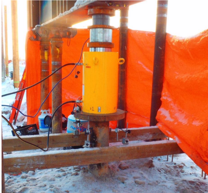
Figure 3.4 - Load Cell and Dial Gauge Set Up
