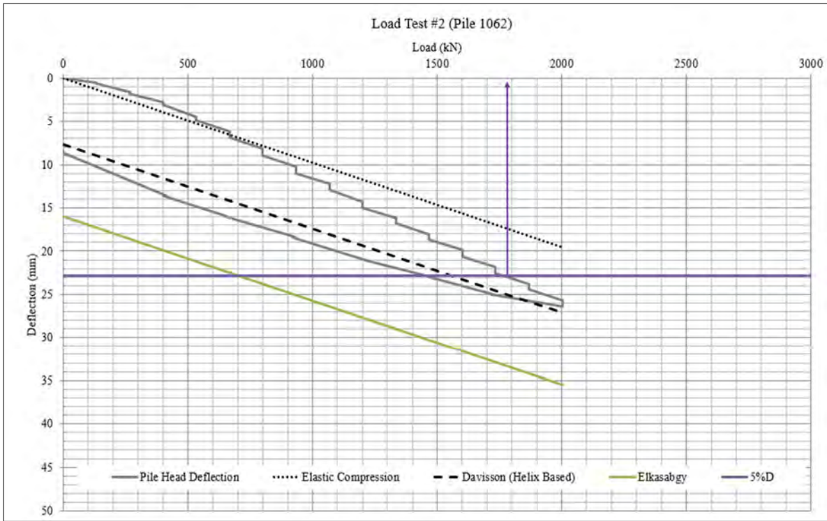
Figure A2a. Load Test Interpretation
