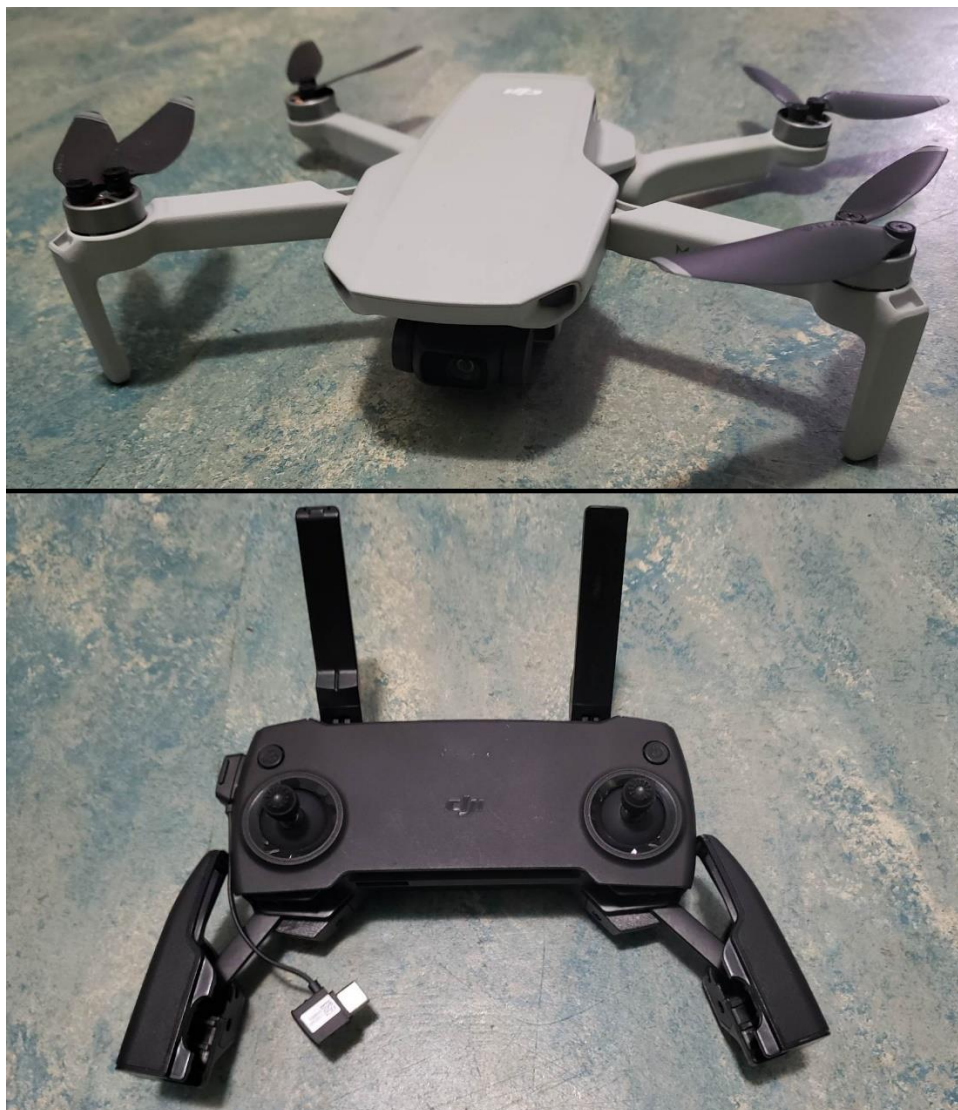
Figure 11. DJI Mavic Mini (first generation) micro-RPA (top) and controller (bottom). A phone or tablet is connected to the controller during flight, displaying the perspective of the Mavic Mini during flight.
