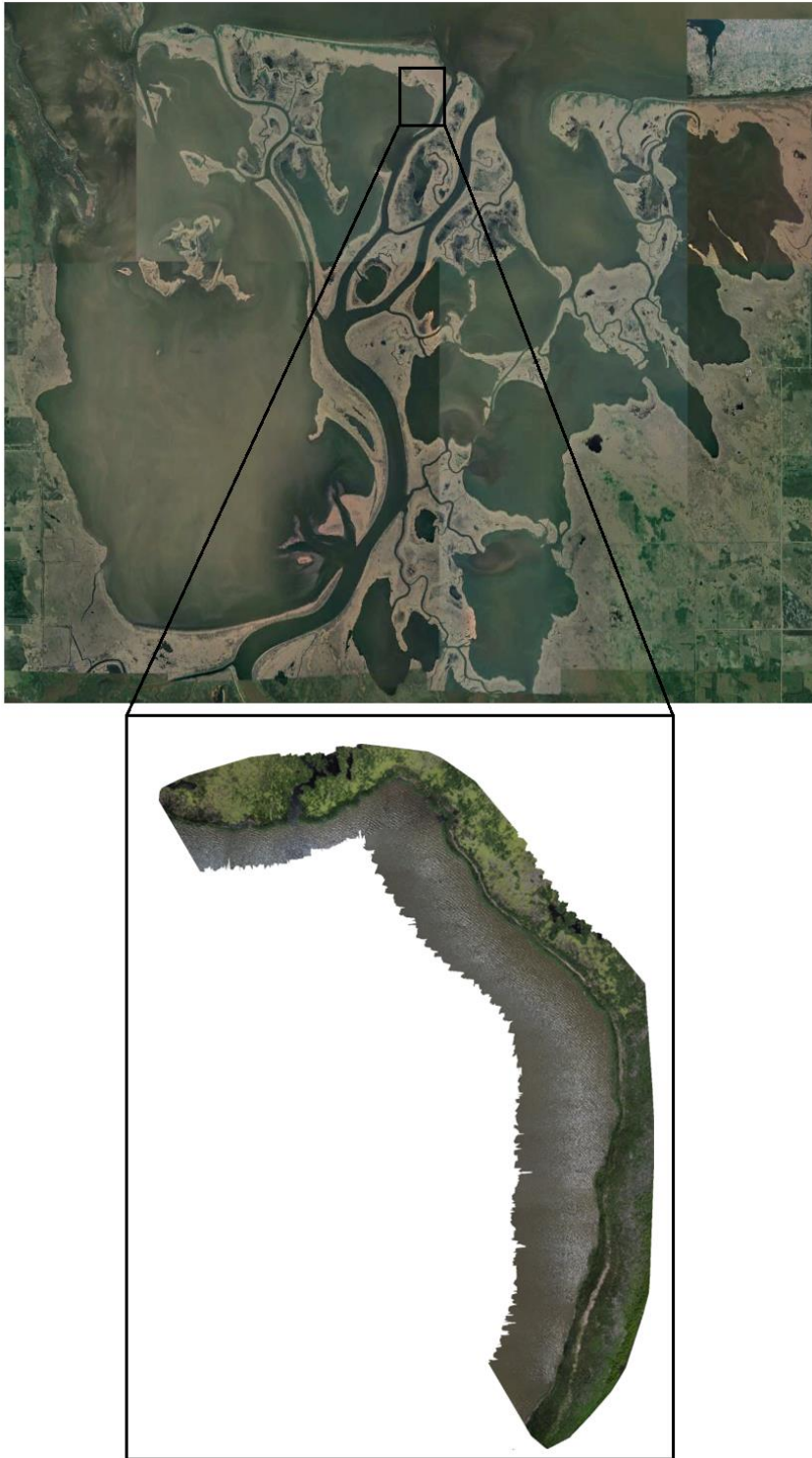
Figure 28. The first corridor mapping practice orthomosaic that I made on a scale that is comparable to the final orthomosaics that I used in my analysis ( > 10 ha). Photos taken July 12, 2020, using a DJI Mavic Mini (first generation). Images stitched together using WebODM. Area depicted is Hardman Lake.
