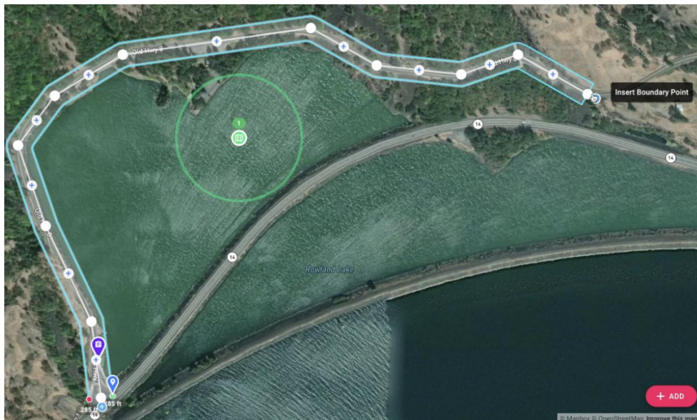
Figure 3. Example of a corridor mapping mission, consisting of two passes along a curved strip. The flight path is depicted in light blue. Reproduced from https://support.dronelink.com/hc/en-us/articles/14090648504083-Linear-Corridor-Mapping .
