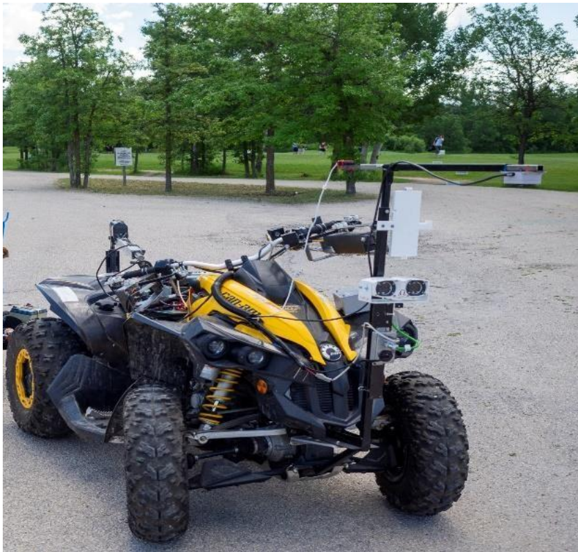
Fig 3. 2: An ATV with camera mounted on the field plot
