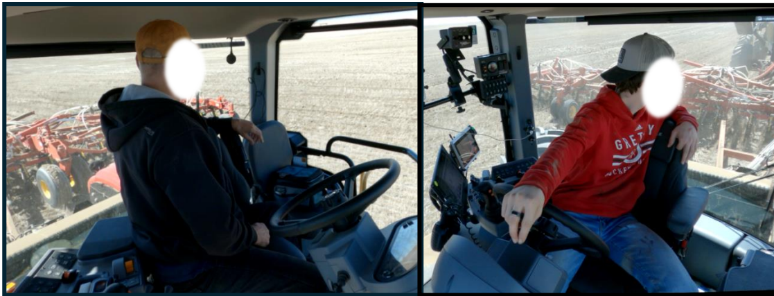
Figure 1. Footage of operator 2 and 3 while having their back twisted and monitoring the rear implement.
