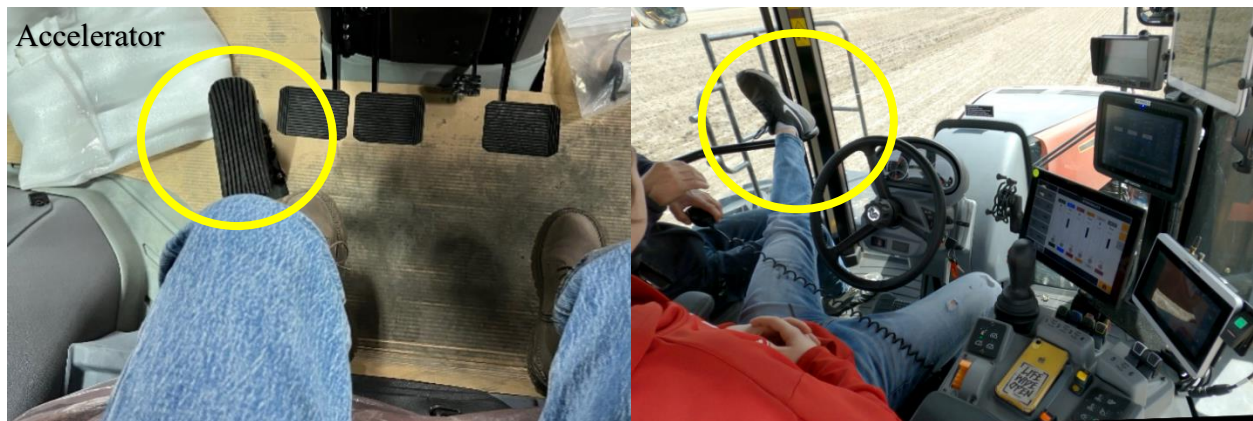
Figure 11. The placement of the accelerator pedal causes discomfort and leads to improper foot positioning.
