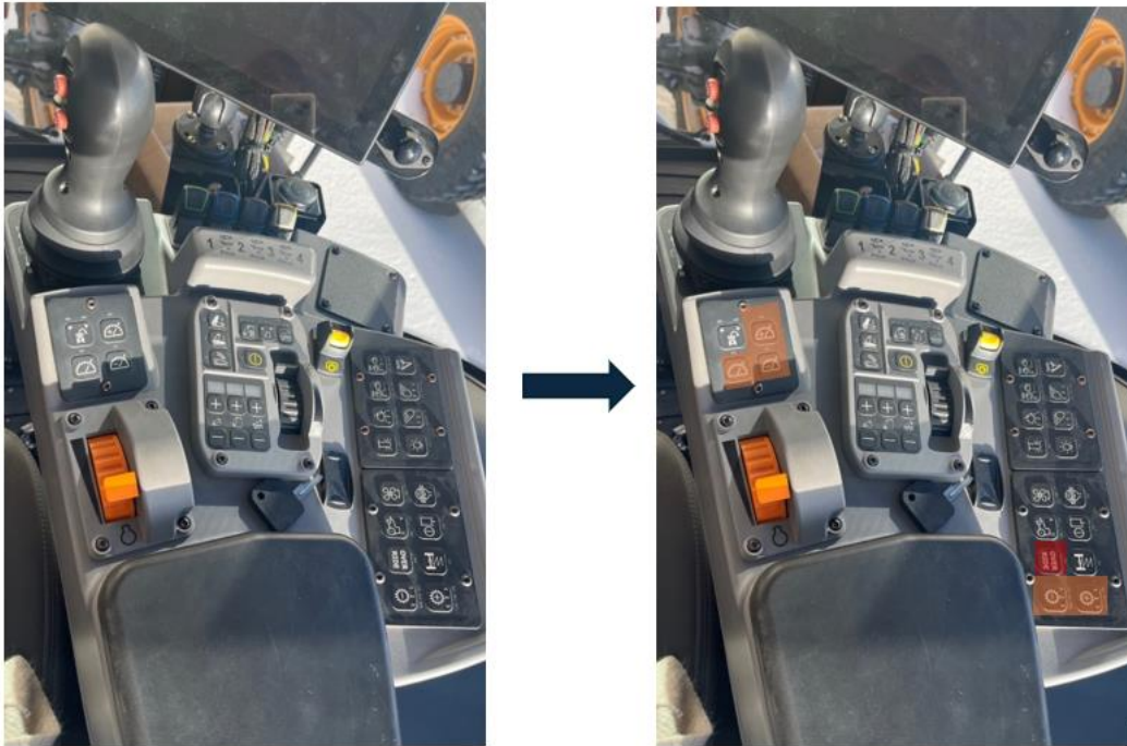
Figure 7. On the left, minimal color coding of the armrest. On the right, color-coded buttons for the engine and transmission.
