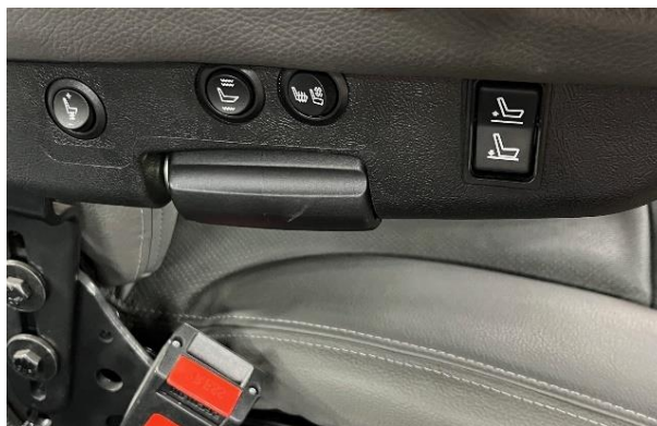
Figure 12. The placement of seat adjustments on the side of the armrest hinders visibility.
