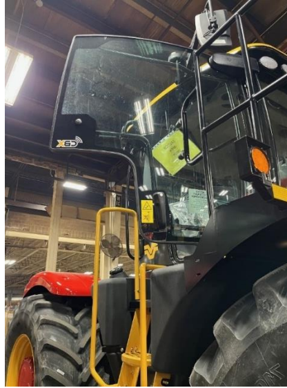
Figure 13. The doorknob's position caused the door to swing towards the operator's face, creating a safety hazard.
