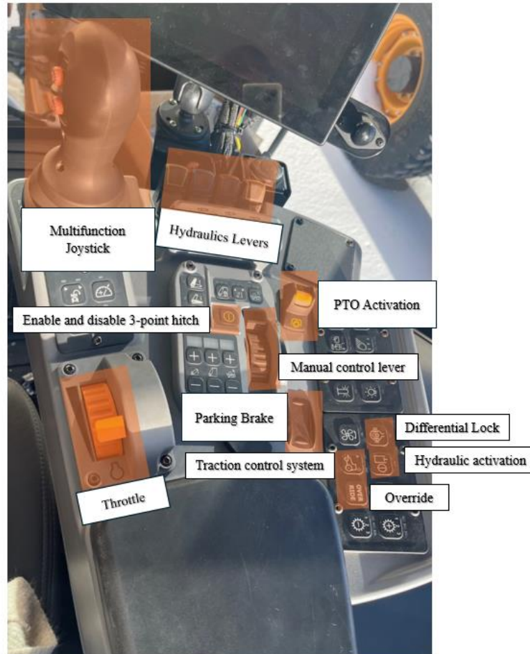
Figure 36. The selected physical buttons to retain on the armrest of a semi-autonomous tractor.
