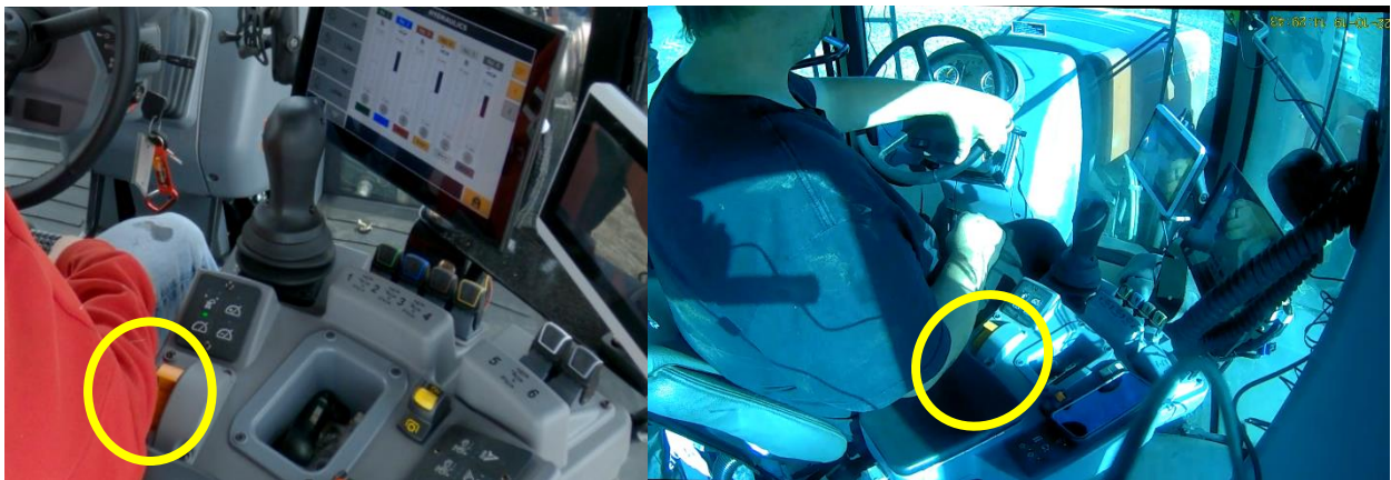
Figure 10. The forearm being positioned very close to the engine throttle poses a safety risk.
