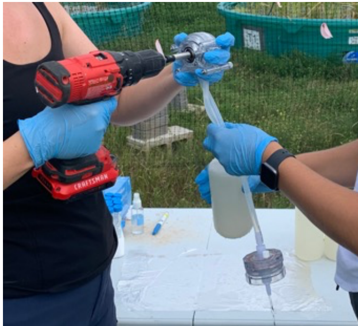
Figure 2.4: The “DIY” peristaltic pump filtering system used to sample eDNA within water samples from the mesocosms.
