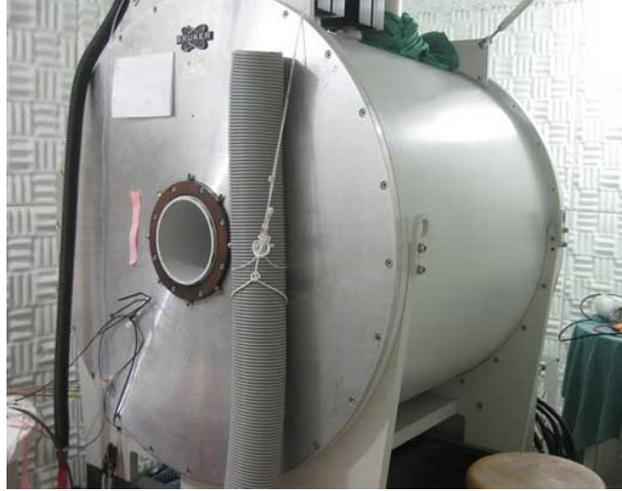
Figure 3.2: The 7T 21 cm Bruker Avance III MRI System used to collect *in vivo* and *ex vivo* images.
