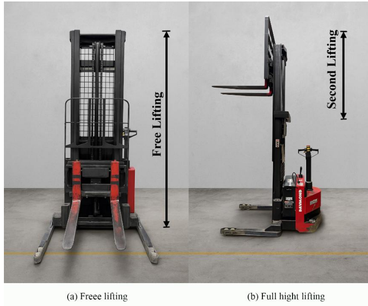
Figure 2-6: Forklift lift function: (a) Free lift zone, and (b) Full height lifting.
