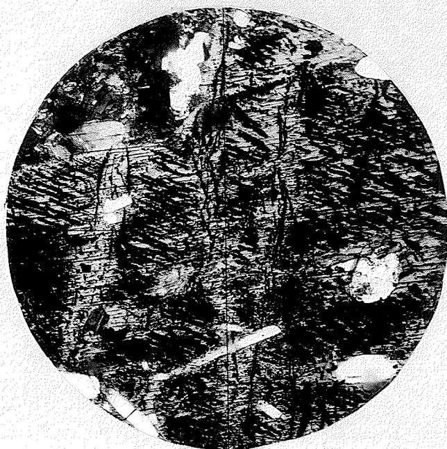
Figure 7. Photomicrograph of magnetite lamellae in hornblende, specimen CG 6-6 (plane polarized light). Diameter of field view is 2.8 millimetres.
