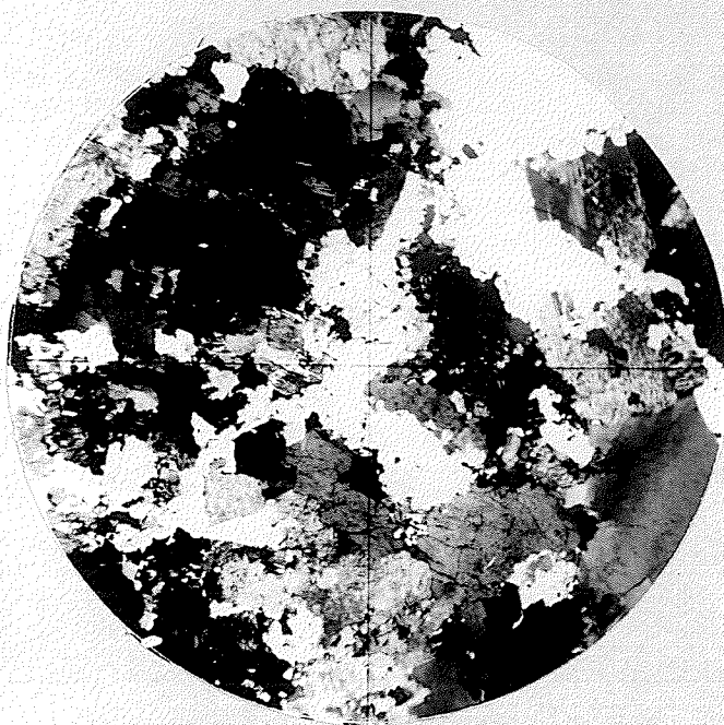
Figure 11. Pronounced development of granophyric (?) quartz in granite. Quartz appears white. Specimen CG 2-2 (crossed nicols). Diameter of field of view is 7 millimetres.
