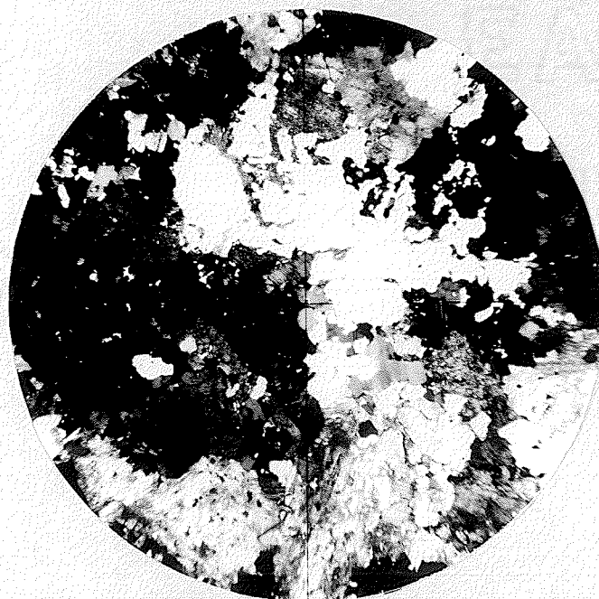
Figure 12. Extreme development of granophyric (?) quartz in granite. Quartz appears white. Specimen CG 6-22 (crossed nicols). This is the same specimen as figure 10. Diameter of field of view is 7 millimetres.
