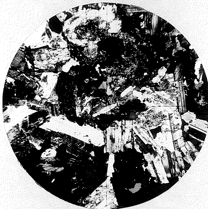
Figure 5. Photomicrograph of typical gabbro, specimen CG 9-21 (crossed nicols). Diameter of field of view is 7 millimetres.
