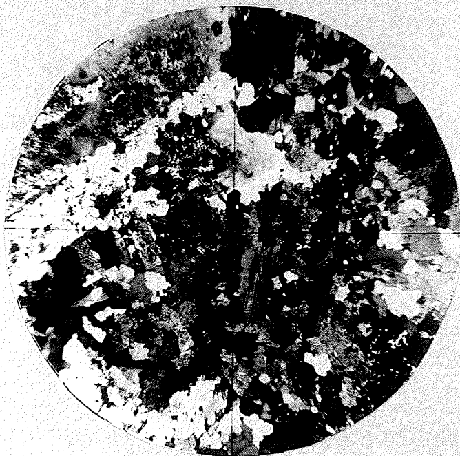
Figure 9. Photomicrograph of a basal transition rock showing granophyric (?) quartz-feldspar intergrowth. Quartz appears white. Specimen CG 6-14 (crossed nicols). Diameter of field view is 7 millimetres.
