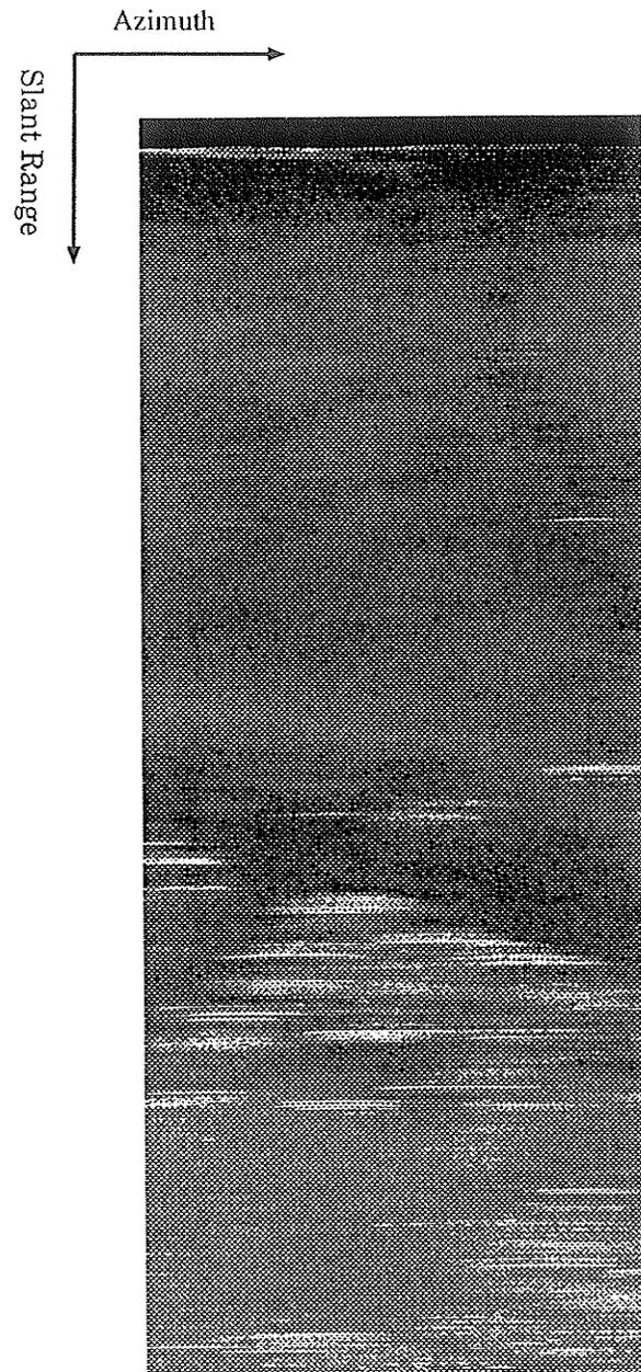
Figure 5.9: Raw airborne SAR signal which was acquired near Ottawa, Canada, using CCRS's C-band airborne SAR system on August 10, 1990. Operating mode was the nadir half-swath mode in HH-polarization. Flight path direction is from top left to top right in this image.
