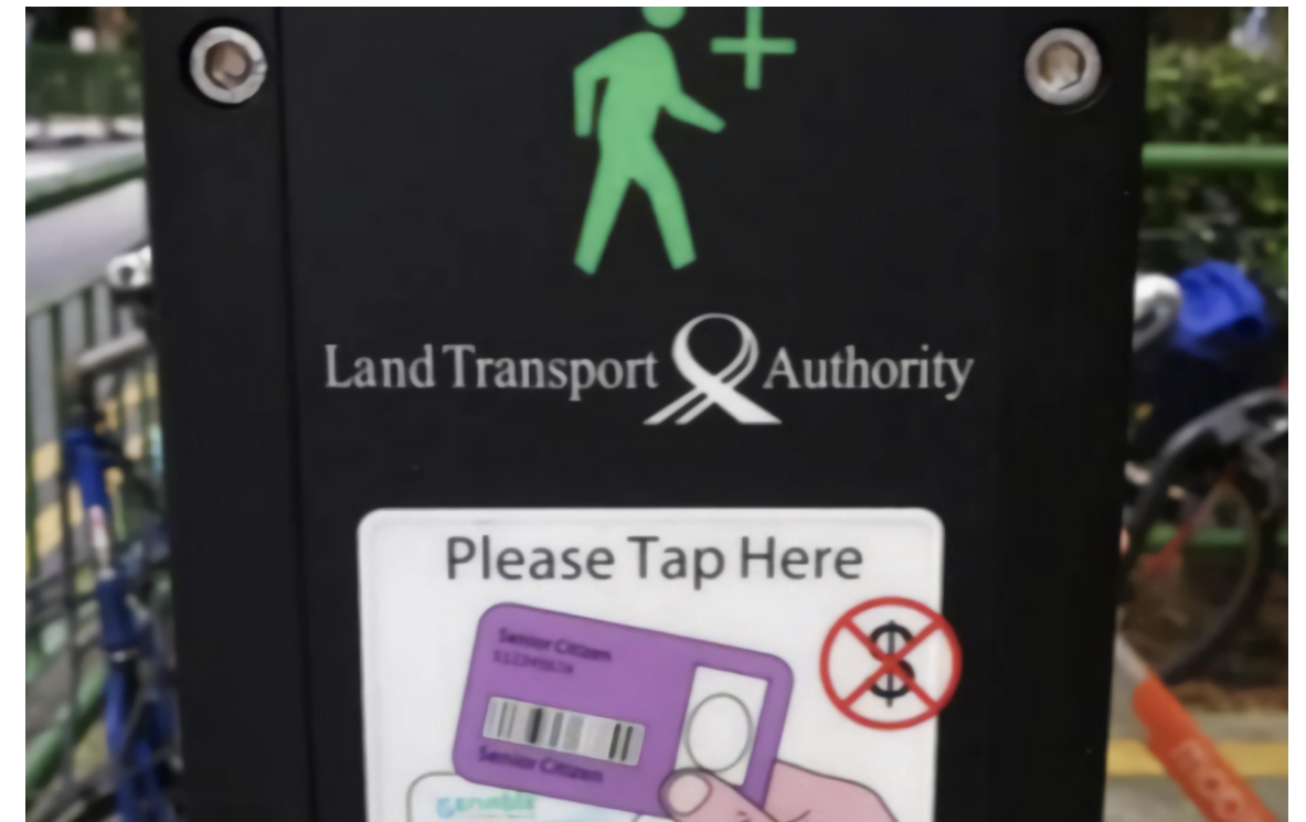
Figure 4-20: Card readers to extend traffic lights for old pedestrians.
