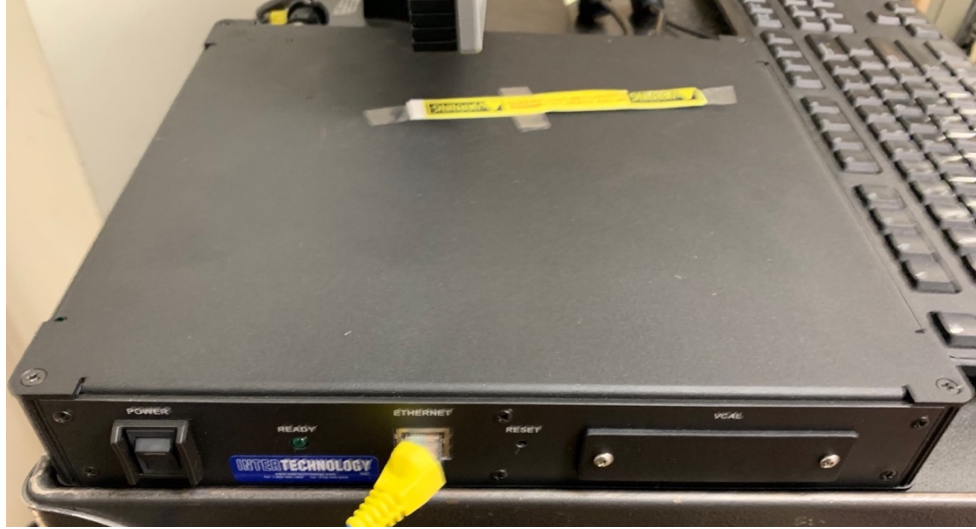
Figure 3-10: MicroMeasurements Strain Smart 8000 Data Acquisition System
