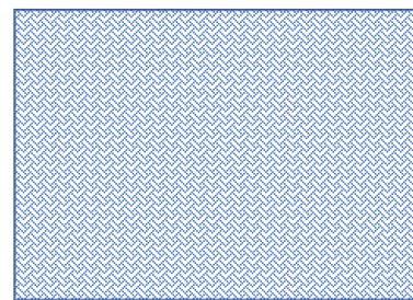
Figure 1-3: Woven continuous fibre reinforcement architecture.
