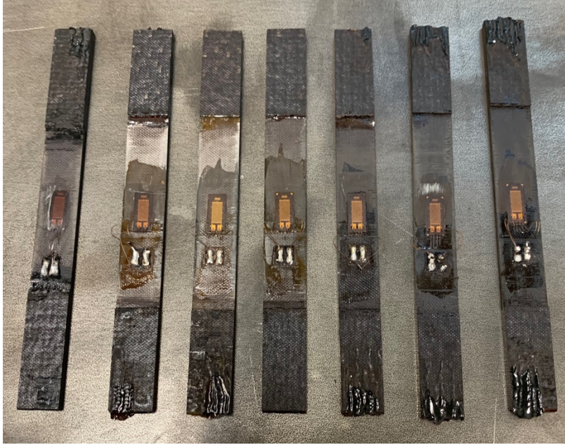
Figure 3-7: Seven prepared samples after polishing of the edges and bonding of the strain gage.
