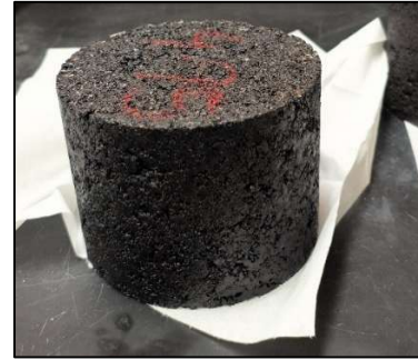
(a). Conditioning of the Mix for Two Hours at 140 °C (b). Sample After Gyratory Compaction
