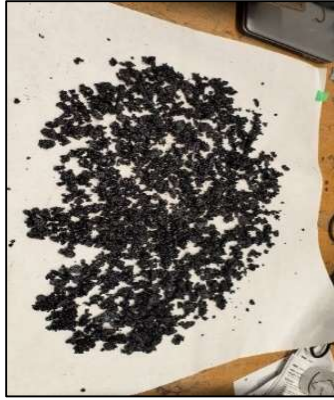
(a) Loose sample for G_{mm} (AASHTO T209,2014)
