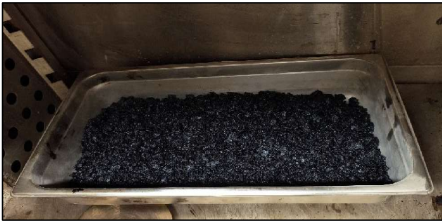
(a). Conditioning of the Mix for Two Hours at 140 °C (b). Sample After Gyratory Compaction
