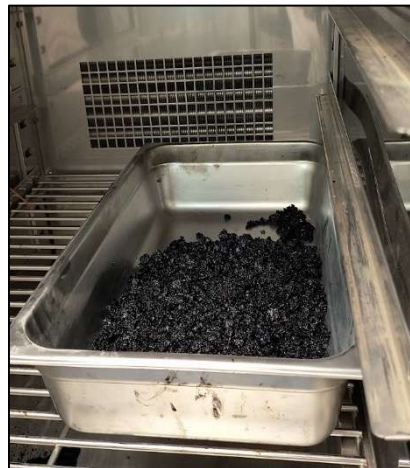
(b) Curing of Mix at 60^\circ\text{C} for 24 hours
