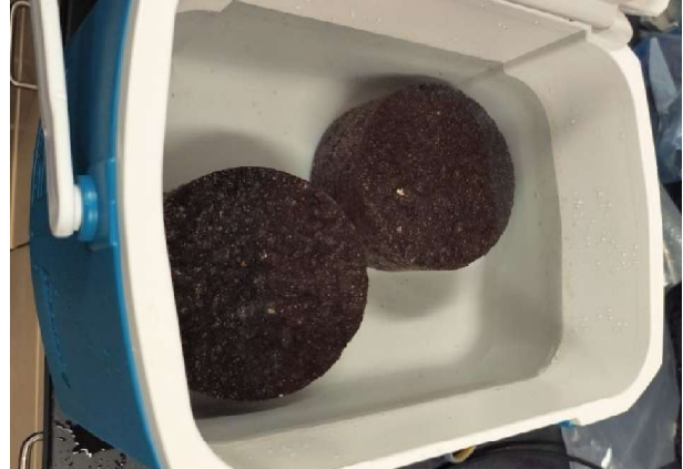
(a) Wet subset in Water Bath at 60°C for 24 hrs (b) Wet subset in water bath at 25 °C for two hrs
