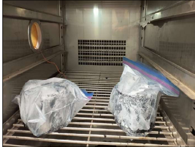
(b) Specimen conditioning at -18^{\circ}\text{C} for 16 hours
