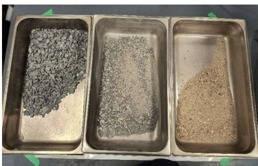
(a) Aggregate proportion for Laboratory Mix (b) Mixing aggregates with binder at 155 °C
