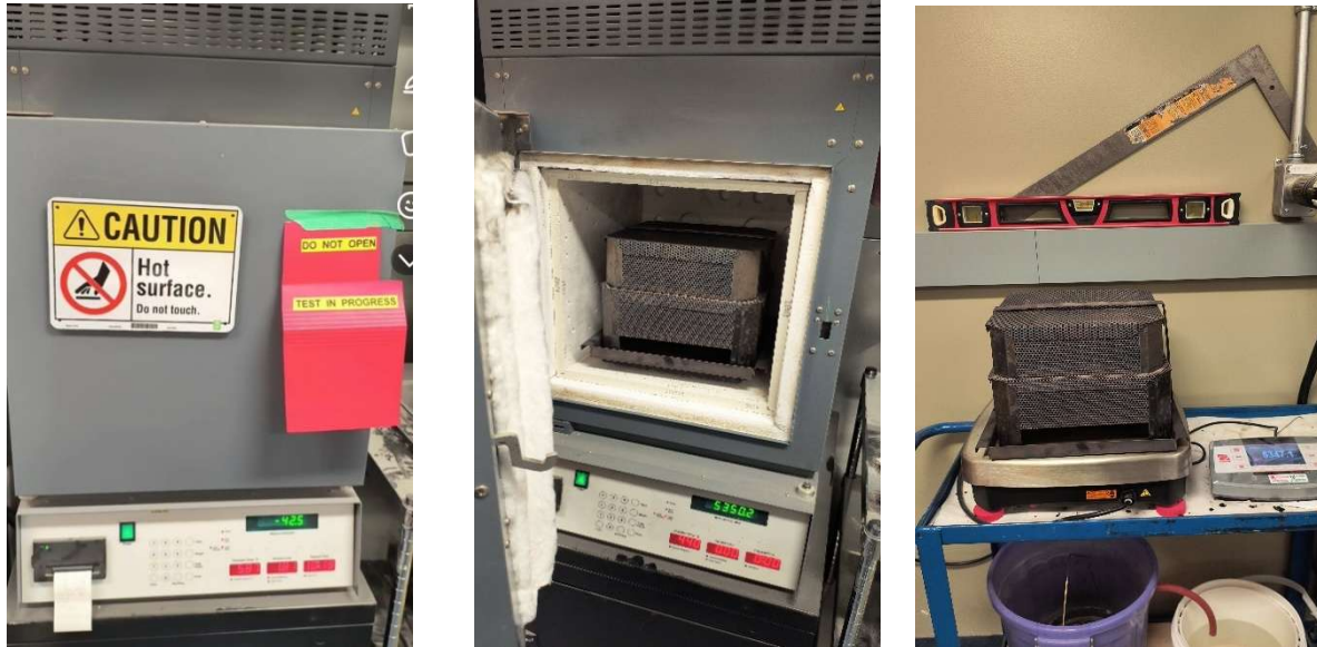
(a) Test Setup in Chamber (b) Ignition Trays with Loose Mix (c) Find Mass of Recovered aggregates (uncalibrated)
