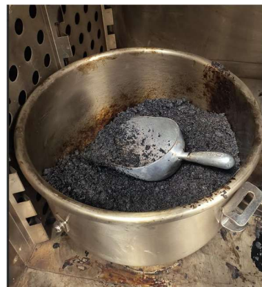
(b) Heating the mix to extract HWTT sample
