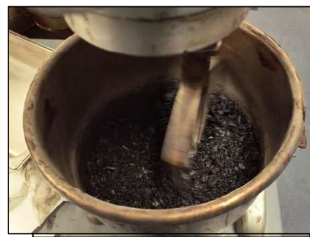
(a) Aggregate proportion for Laboratory Mix (b) Mixing aggregates with binder at 155 °C
