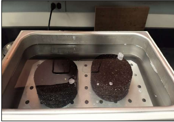
(a) Wet subset in Water Bath at 60°C for 24 hrs (b) Wet subset in water bath at 25 °C for two hrs
