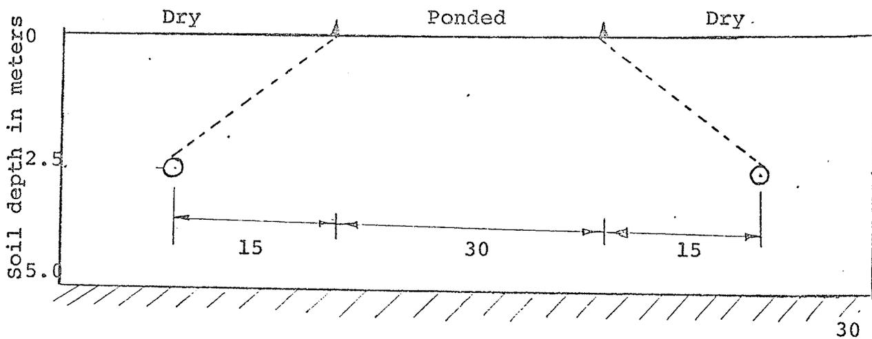
Fig. 17 Reclamation of saline soils by leaching (diking) and tile drainage. (After Luthin, 1950).
