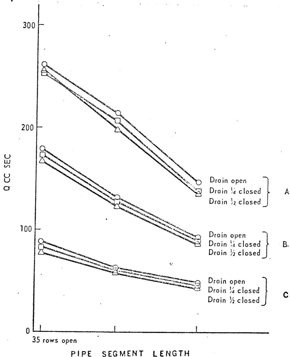
Fig. 15 Effect of pipe segment length on flow into drain. The "35 rows open" is a completely permeable drain perforated with 35 rows of holes. All drains were wrapped with glass fibers. The "drain open" is an empty drainpipe. One fourth and one half closed have weits to maintain the water level at one fourth and one half of drain diameter. A, B, and C = height of water in reservoirs. (after Luthin and Haig, 1972).
