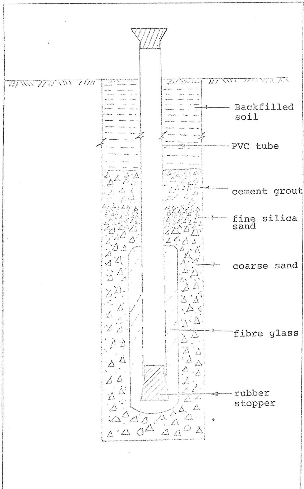
Fig. 21 Design of piezometer used to measure ground water hydraulic head.
