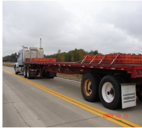
(b) 5-Axle Semi Trailer Loading
