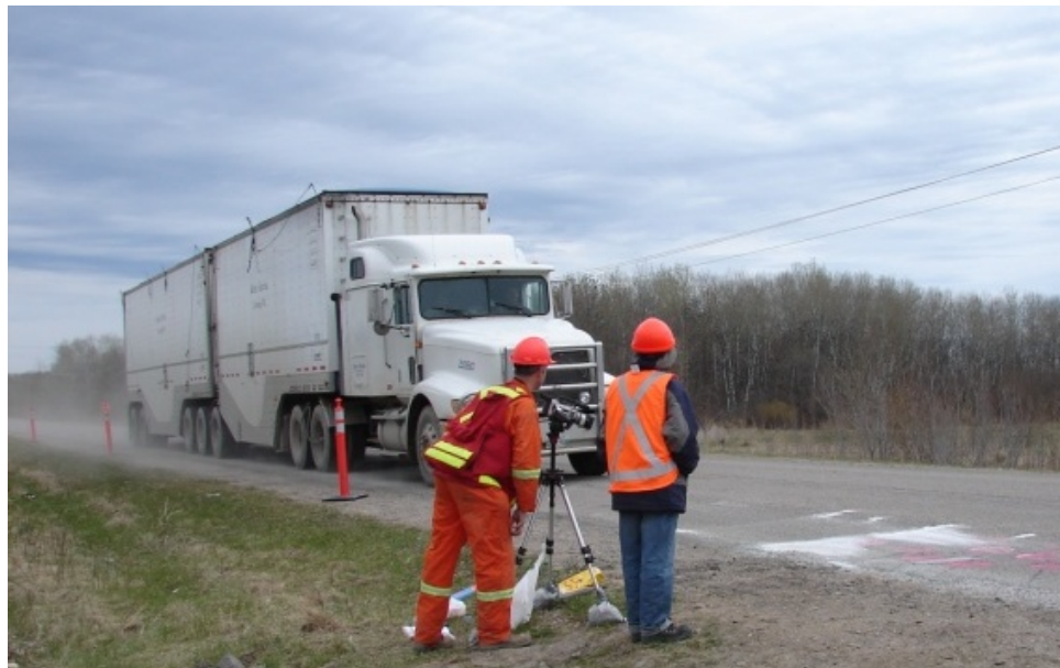
Figure 4.6: B-Train Trafficking Over Pavement Sensors at Manitoba Site
