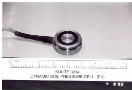
(c) Dynamic Soil Pressure Cell (PK)
