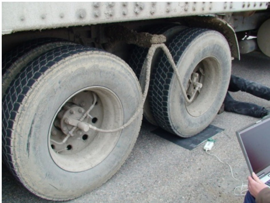
Figure 4.8: Tire-Pavement Contact Pressure Distribution Testing with I-Scan Pressure Mat at Manitoba Test Site
