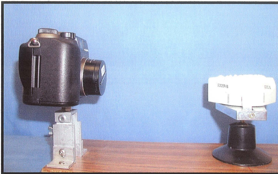
Figure 3.4 Adjustable photographic apparatus used to digitally record right and left curve of Spee from plaster study models.
