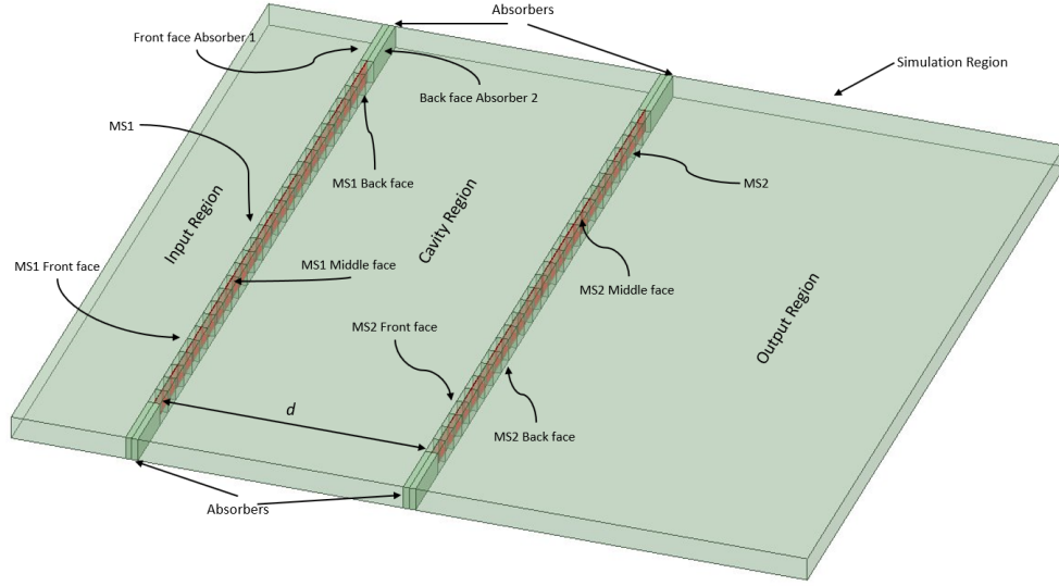
Figure 4.1: A complete setup of a cascaded metasurface system with surface impedance specifications on the three layers of each unit cell. The two dielectric substrates are Rogers RO3010 which are bonded by Rogers 2929 bondply.
