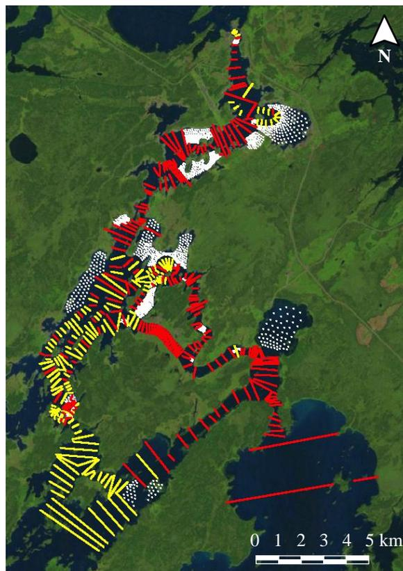
Figure 4.1. Summary of available original (red), proxy (yellow), and estimated flood zone (white) bathymetric data
