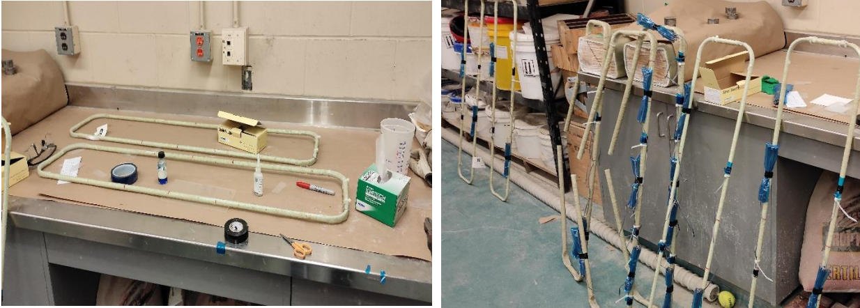
(E) Preparation of bars for installation of strain gauges
