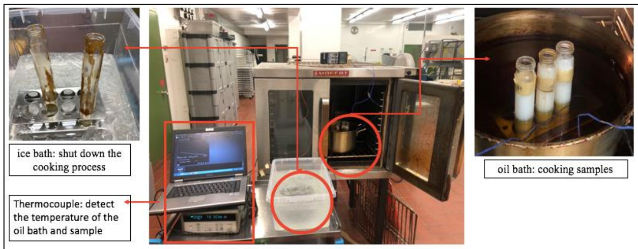
Figure 3.2 Roux cooking apparatus set-up.
