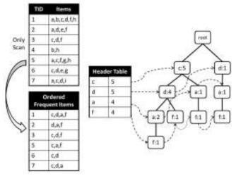
Figure 2. An FP-tree used in the FP-growth algorithm for mining frequent patterns with a minimum support of 3.
