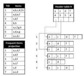
Figure 3. An H-struct used in the H-Mine algorithm for mining frequent patterns with a minimum support of 3.
