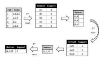
Figure 1. Example run of the Apriori algorithm with a minimum support of 2.
