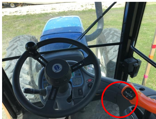
Figure 20 control panel blocked the view.
