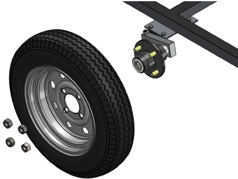
Figure 76: Assembly diagram of the wheel mounting to the hub of the axle
