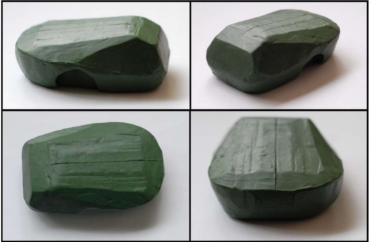
Figure 17: Plasticine model of final body design.
