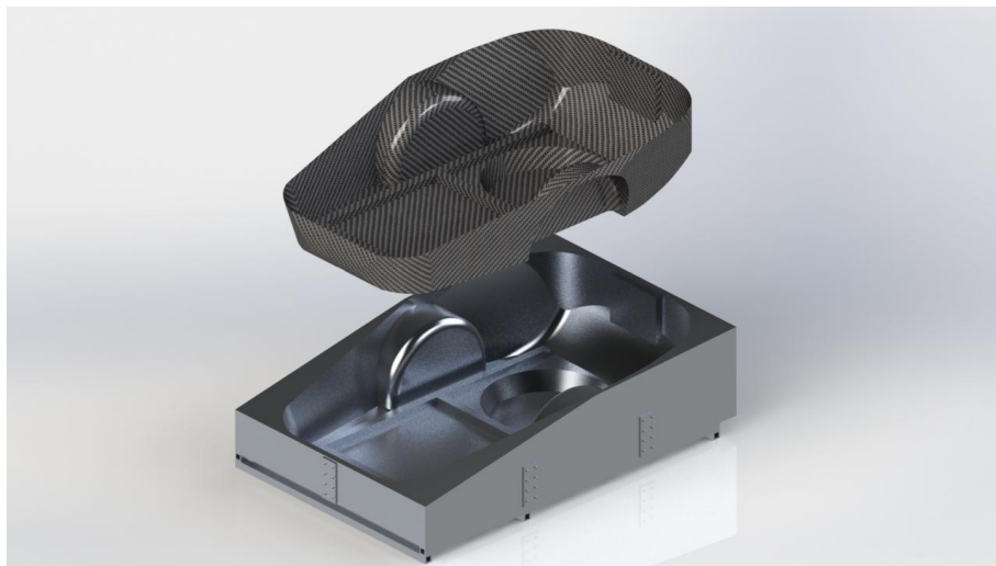
Figure 20: Part removal upon completion of curing
