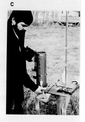
Supply Co., Michigan, U.S.A. (Fig. 5). The original drainage system of the VDB did not allow passage of larger invertebrates from the cylinder and as a result the original cylinders were replaced with a comparable section of PVC 12 cm diameter pipe (2 l volume) which had a 2 cm diameter drainspout located 6 cm from one end. A 16 cm section of 2 cm diameter Tygon tubing was placed on the drain and the flow of water from the VDB regulated with a pinch clamp.
