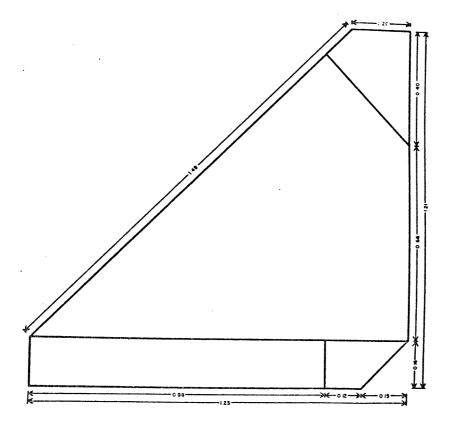
Figure 6. Dimensions of north and south faces of the emergence traps (dimensions in meters).
