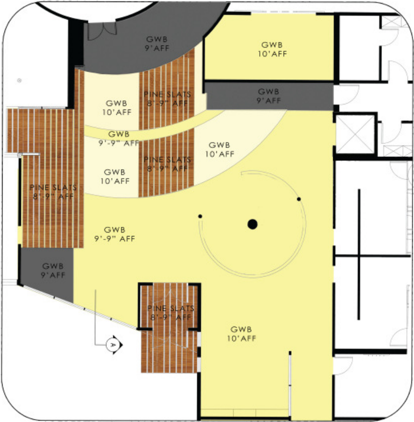
REFLECTED CEILING PLAN
