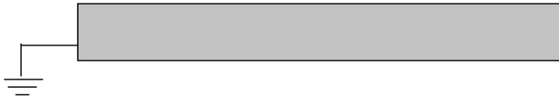
Figure 14: High frequency model for the Field Perturbing Element in ON mode
