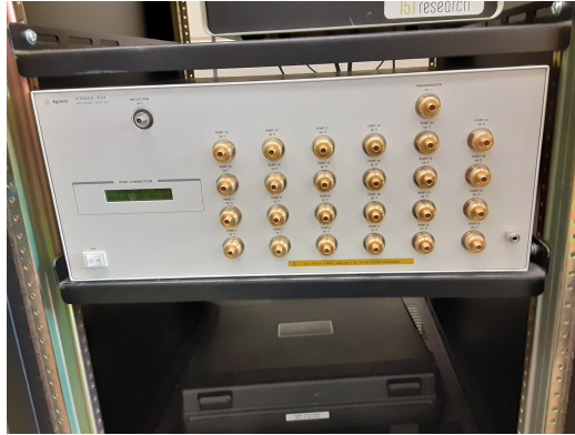
Figure 5: RF switch device used in order to multiplex the VNA ports and feed the 24 port systems
