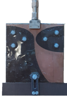
Figure 7: one of the Vivaldi antennas used in [27]
