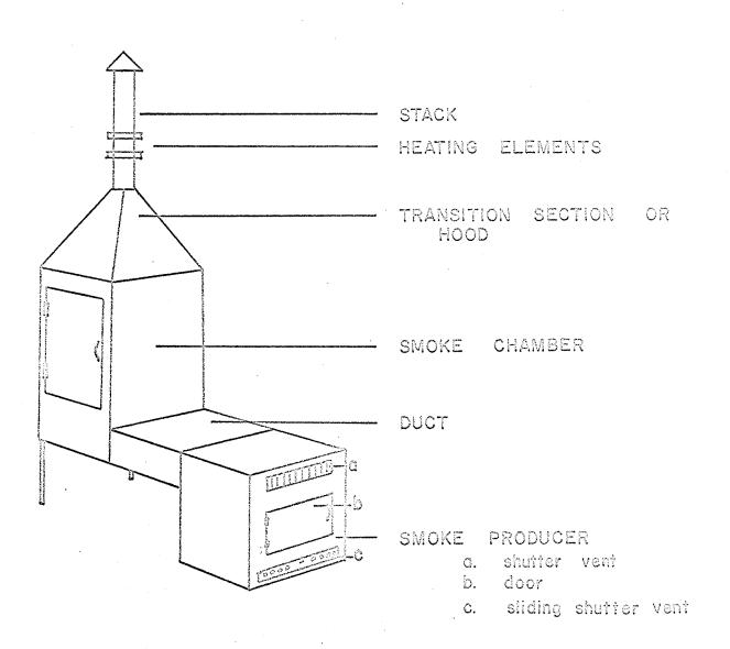
which consisted of two adapters for controlling output of smoke and heat. In addition, two heating elements capable of producing heat up to 550°F were installed in the stack in order to destroy any <u>Salmonella</u> which may escape through the chimney during the smoking process.
